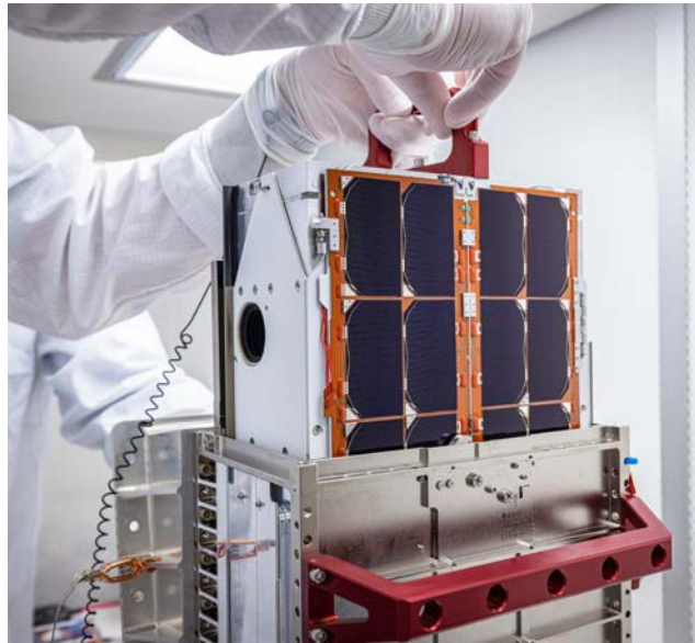
Figure 2. LICIACube in August 2021, prior to its integration on the DART spacecraft. LICIACube is a 6U CubeSat contributed by the Italian Space Agency, with dimensions of 10 cm x 20 cm x 30 cm.
