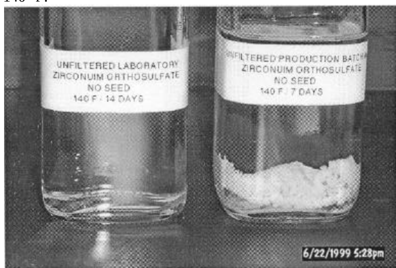
FIGURE I: Laboratory ZOS (left) and Production ZOS (right) solutions stored at 140^{\circ}\text{F} for 14 and 7 days, respectively. Both samples are unfiltered. The laboratory sample showed no signs of deposits.
