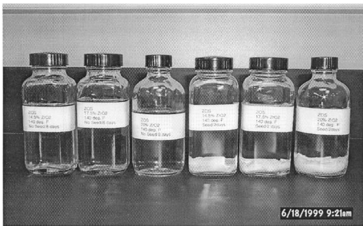
FIGURE 2: Laboratory ZOS samples with and without ZOS scale present as seed crystals and stored at 140° F. Left 3 samples (no seed) are 14.5, 17.5, and 20% ZrO 2 . Right three samples (with seed) for 14.5, 17.5, and 20% ZrO 2 .
