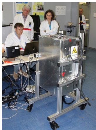
Figure 4.2. LS-NCC fast neutron detector developed by IAEA.
