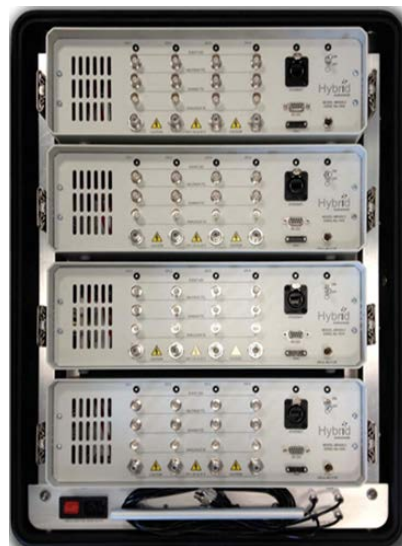
Figure 3.21. Instruments with 4 x 4-Channel Mixed-Field Analyzer by Hybrid Instruments, Ltd.
