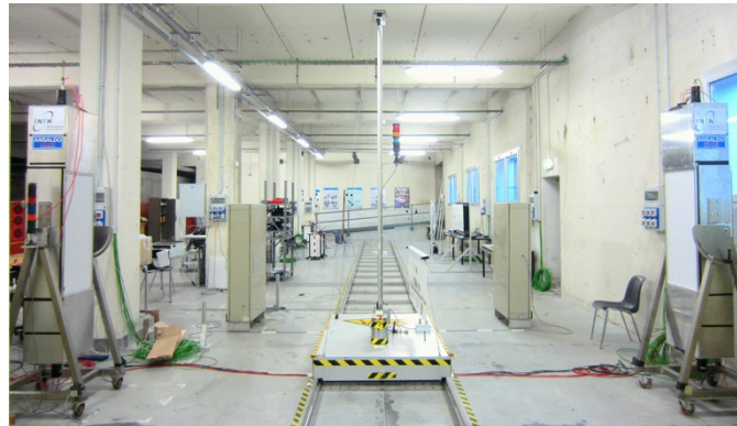
Figure 3.28: The INFN/ANN RPM prototype during the blind benchmark in the ITRAP+10 JRC facility. The trolley, used for testing, is transiting in between the 2 pillars.
