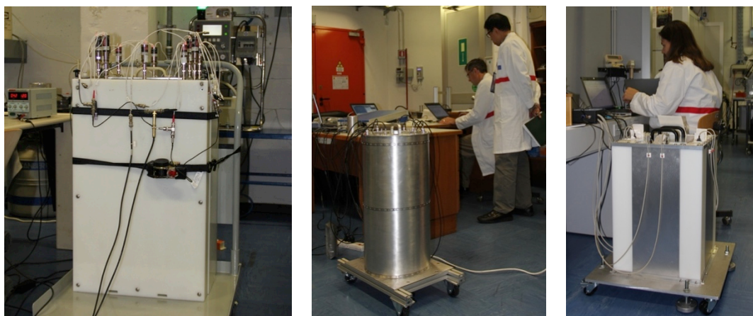
Figure 4.1. (left) GERS-NCC, modified ABUNCL well counter; (center) BCS-based HLNCC well counter developed by PTI; (right) well counter with ^6\text{Li}/\text{ZnS} blades developed by Symetrica.
