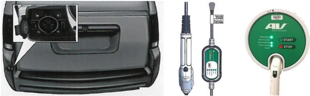
Figure 10: On-board charging port, portable EVSE and stationary EVSE
