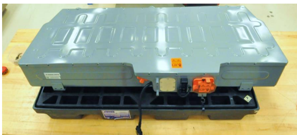
Figure 6: Magna/JCI HV battery as installed in Phase II
