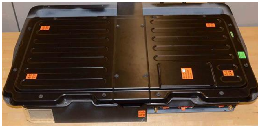
Figure 4: Electroveya HV battery pack as installed in Phase I
