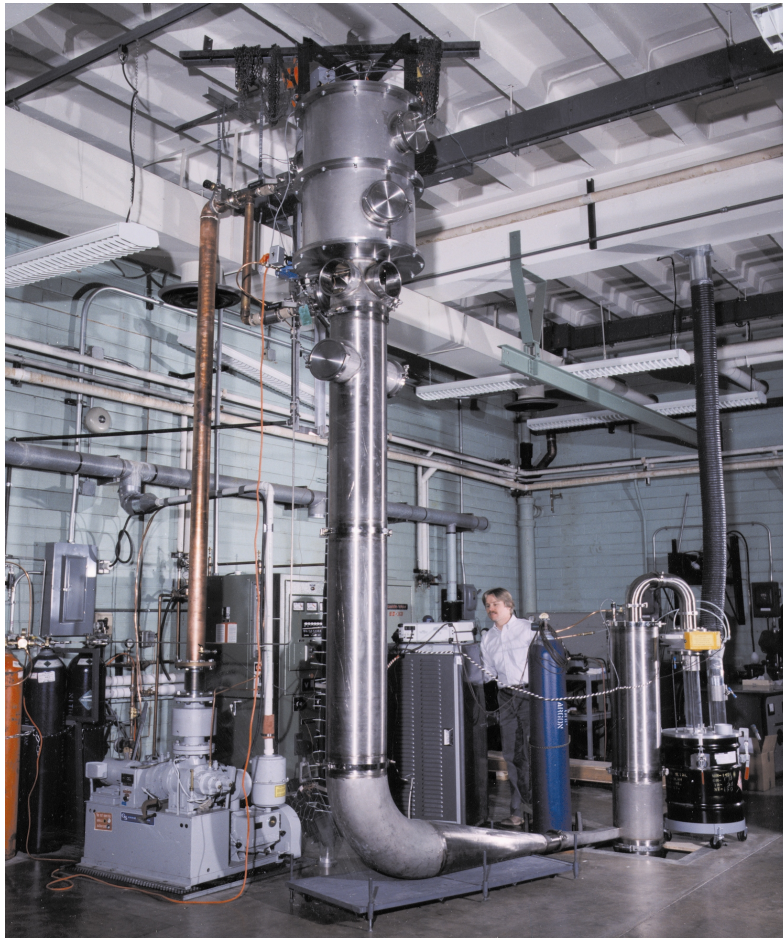
Figure 14. High pressure gas atomizer, Ames Laboratory.
