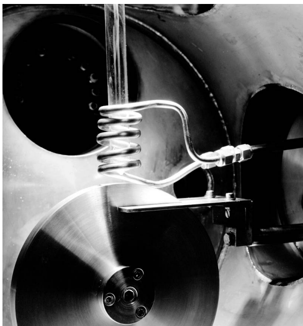
Figure 15. Copper chill block melt spinner, Ames Laboratory.
