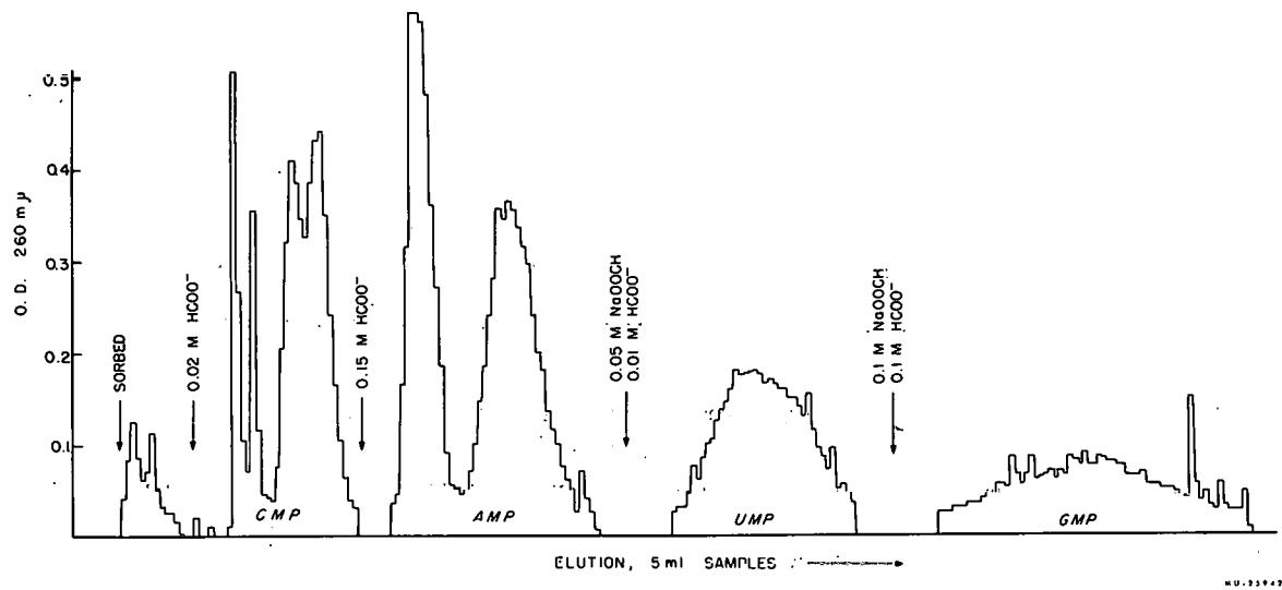
Fig. 10-2. Elution pattern of stroma-RNA nucleotides separated on a formate column, 11 cm  $\times$  1 cm diam, 0.5 ml/min, 5-ml fractions collected.
