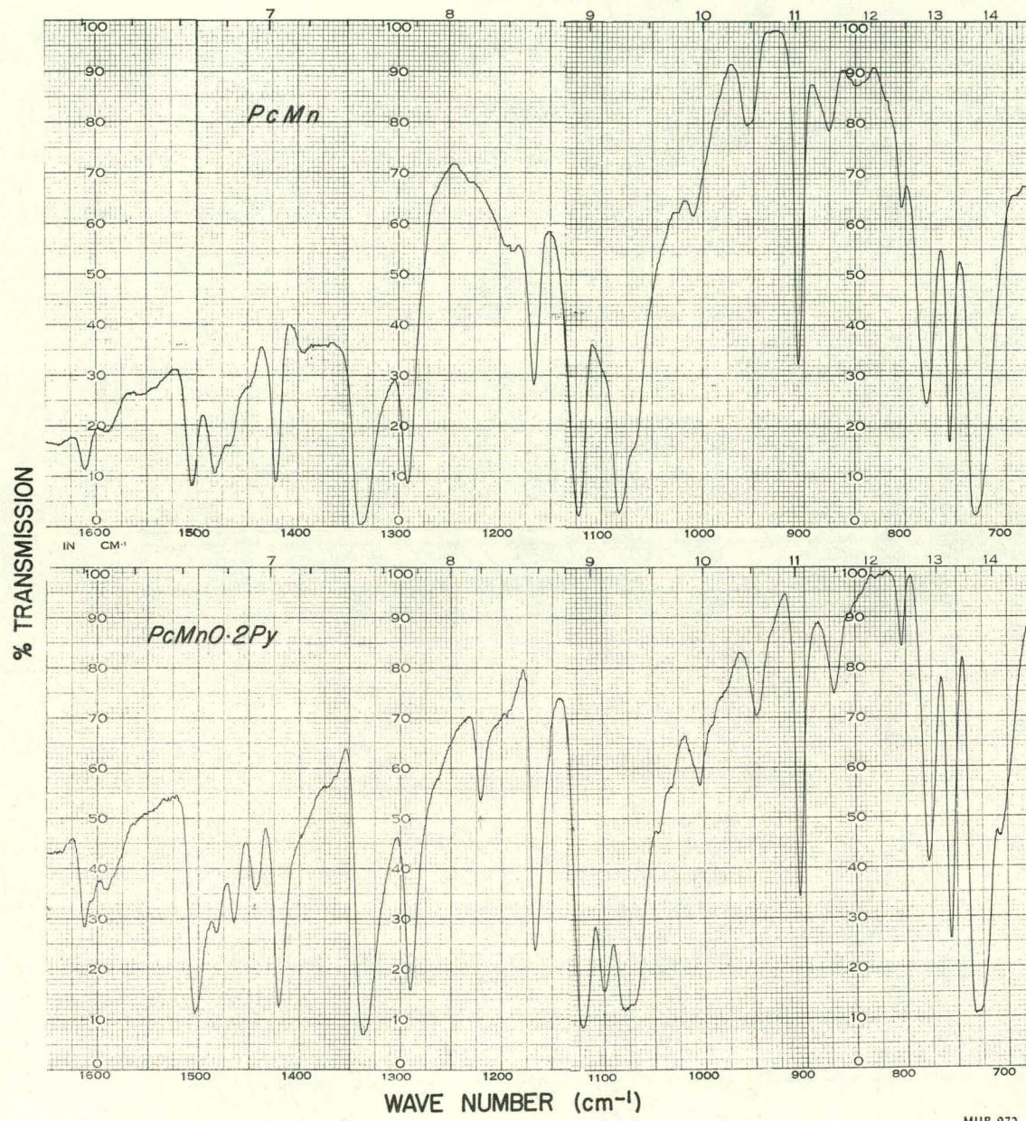
Fig. 13-10. Infrared spectra of  $\text{PcMn(II)}$  and  $\text{PyMnO}\cdot 2\text{Py}$ ,
