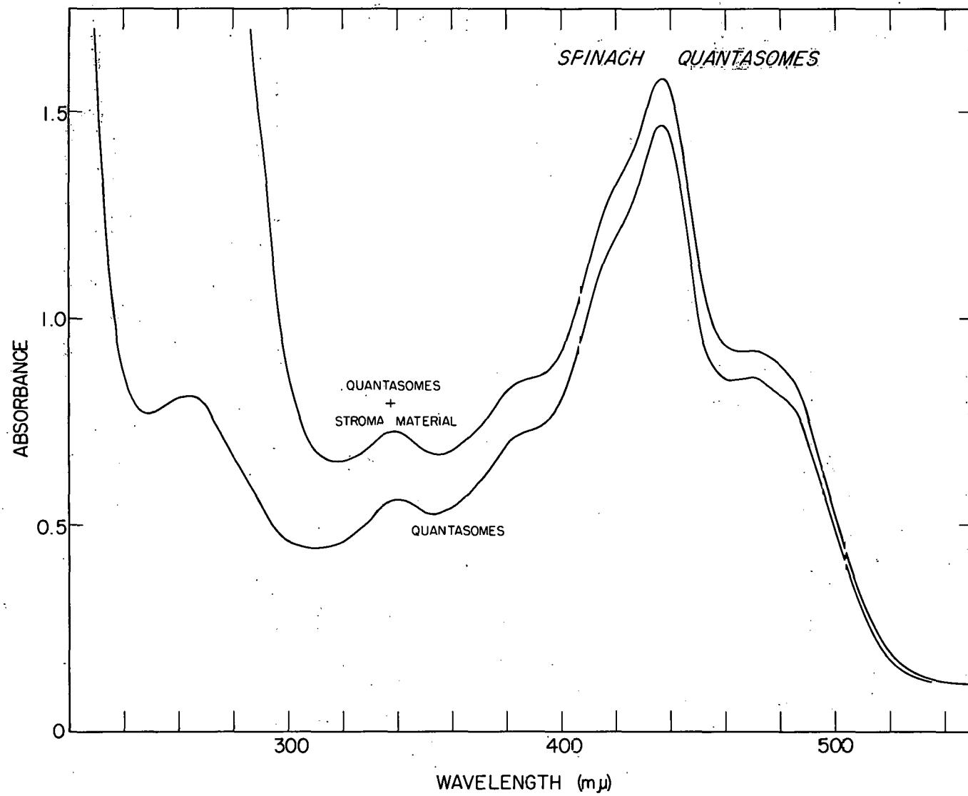
Fig. 11-2. Spinach quantasomes--spectra from 230 to 550 m $\mu$ . Lower curve: quantosome precipitate resuspended (same as Fig. 11-1). Upper curve: quantasomes plus stroma material; supernatant from centrifugation at 145,000 g. The curves were normalized at 678 m $\mu$  (region not shown).
