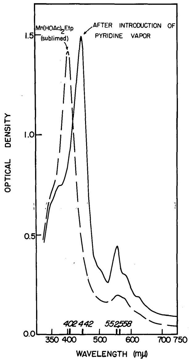
Fig. 13-5. Spectrum of etioporphyrin I di(acetic acid) manganese(II) in the solid state. Lower curve, sublimed in vacuo; upper curve, after the introduction of pyridine vapor.
