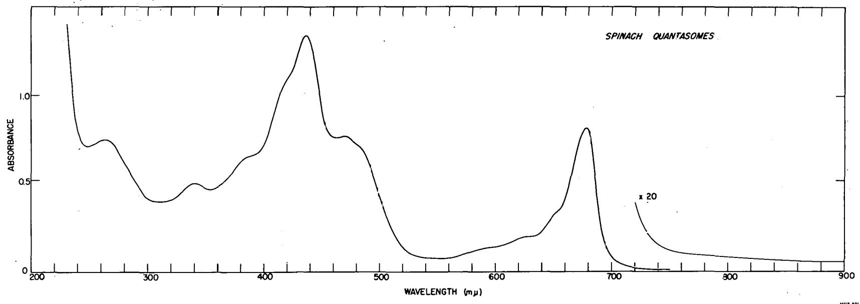
Fig. 11-1. Spinach quantasomes--spectrum from 230 to 900 m $\mu$ . Sample prepared from sonicated spinach chloroplasts; precipitate between 45,000 g and 145,000 g resuspended and resonicated; supernatant from subsequent 20,000 g centrifugation. Curve at right represents 20-fold greater concentration.
