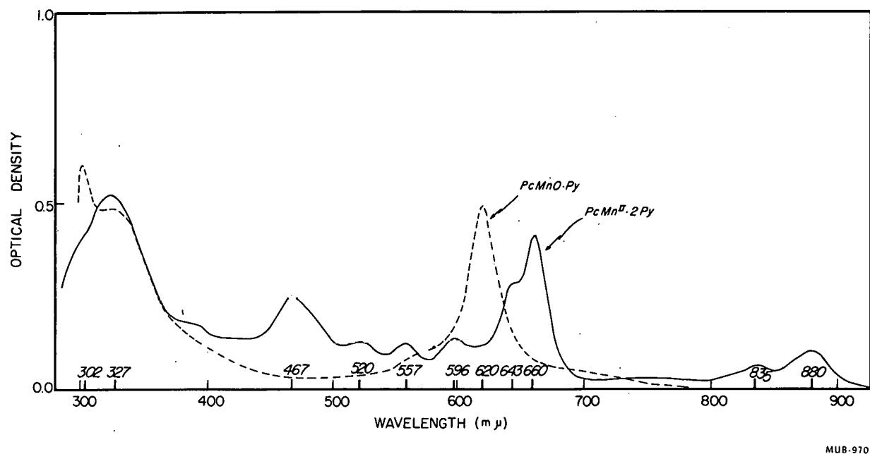
Fig. 13-4. Spectra of Mn(II)Pc·2Py and the oxidation product in pyridine solution.
