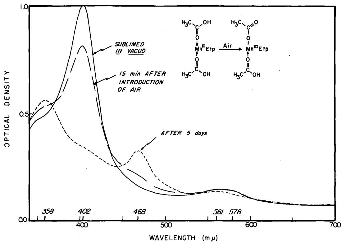
Fig. 13-7. Oxidation of the solid etioporphyrin I di(acetic acid) manganese(II) in air.
