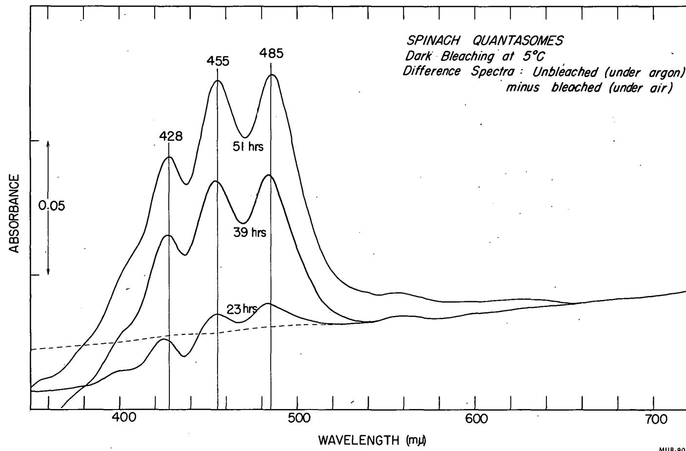
Fig. 11-3. Dark bleaching of spinach quantasomes--difference spectra from 350 to 720 m $\mu$ . Samples prepared from sonicated spinach chloroplasts; precipitate between 45,000 g and 145,000 g resuspended. Difference spectra recorded by using Cary Model 14 spectrophotometer, slide-wire corresponding to full-scale absorbance of 0.1; sample beam, suspension stored under argon; reference beam, suspension stored under air; both kept in dark at 5°. Initial absorbance 1.0 at 678 m $\mu$ .
