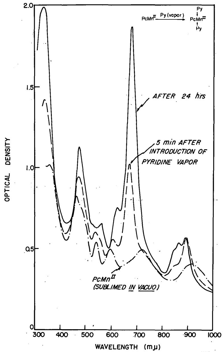
Fig. 13-1. Effect of coordination of pyridine on the visible and uv spectra of phthalocyanine manganese(II).
