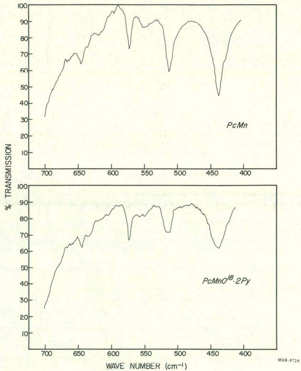
Fig. 13-11. Infrared spectra of  $\text{PcMn}(\text{II})$  and  $\text{PyMnO} \cdot 2\text{Py}$ , CsI region.
