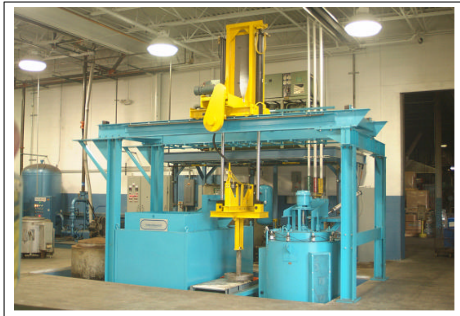
Figure 5. New Batch IQ System With 1,900-gallon Water Tank
