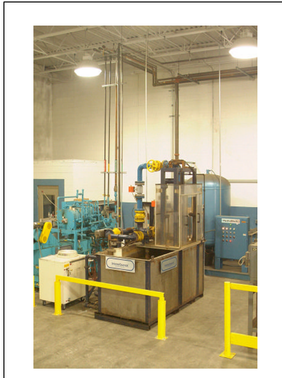
Figure 4. High-Velocity Single-Part Quenching IQ System and Shaker Hearth Furnace with IQ 190-gallon Water Tank
