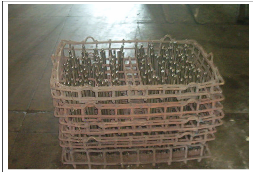
Figure 21. Production Load with Lawnmower Tractor Shaft
