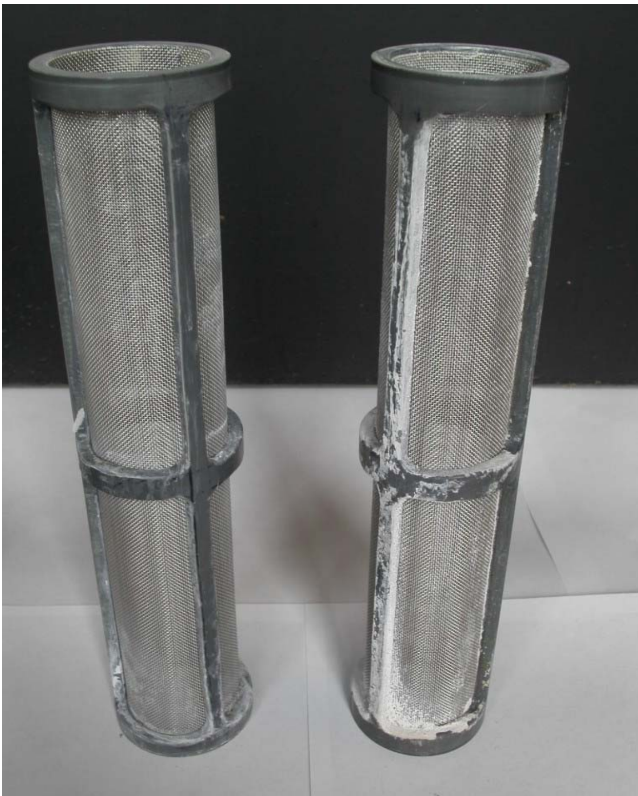
Figure 29. View of stainless steel mesh tube used as spargers in newly designed ASH units after field tests: left – after absorption; right – after stripping.
