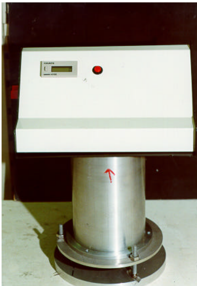
Figure 28. Photograph of the sensor head and control box of the UV photoelectron ion detector.
