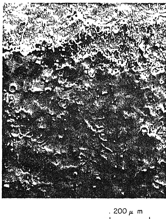
Figure 12. Surface of chromium-carbide coating on type 316 Type stainless steel after 1000 rubbing cycles against 5.56 mm WC sphere.
