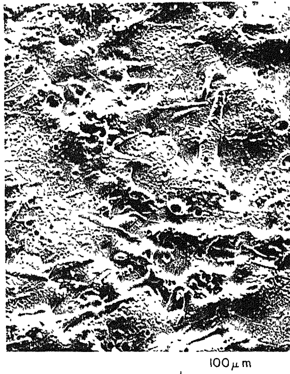
Figure 4. Surface appearance of ESD coating using electrode of 85% \text{Cr}_3\text{C}_2 , 15% Ni with argon gas on type 316 stainless steel.
