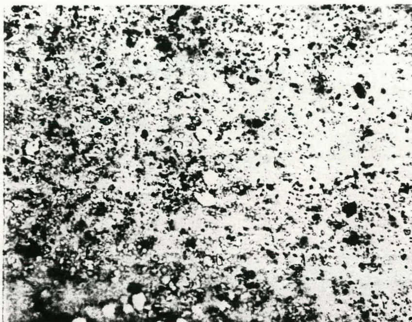
Figure 1. Sample ASH-A (226); slightly uncrossed polars; 263X. Large white particles are clay-coated quartz fragments; fine, gray background particles are mostly clays.
