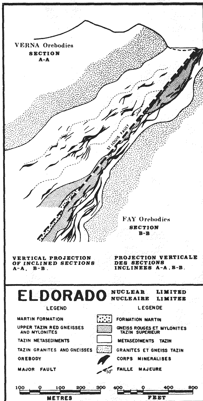
Figure 10. Projection of footwall and hanging wall mineralization onto a cross section, Beaverlodge Operation, Eldorado Nuclear, Canada (from Little et al, 1972).
