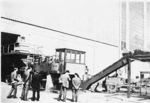
Fig.7 Metal scrap baling equipment and conveyor to a truck loading platform. Sebastian on left, Arley on right
