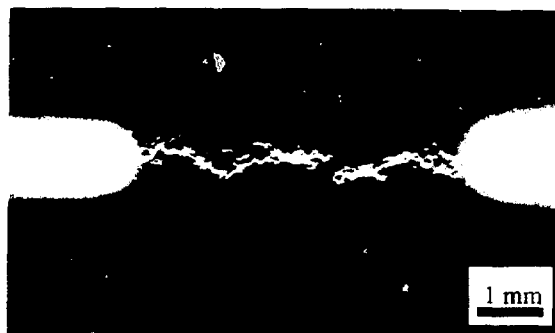
Figure 2. Radiograph of a nearly identical sample as the one from fig. 1 tested at 500°C and interrupted at 0.4 x (max. stress) after the sample had already passed the max. stress.
