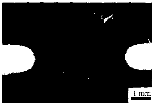
Figure 1. Radiograph of an axisymmetric notched copper sample tested at 500°C and interrupted at 0.75 x (max. stress) while the stress was still increasing.
