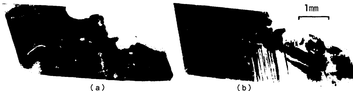
Figure 1. Comparison of neutron (a) ( \lambda = 1.7\text{\AA} , g = \bar{3}21 ) and white beam X-ray (b) ( \lambda = 0.9\text{\AA} , g = 220 ) topographs, respectively.
