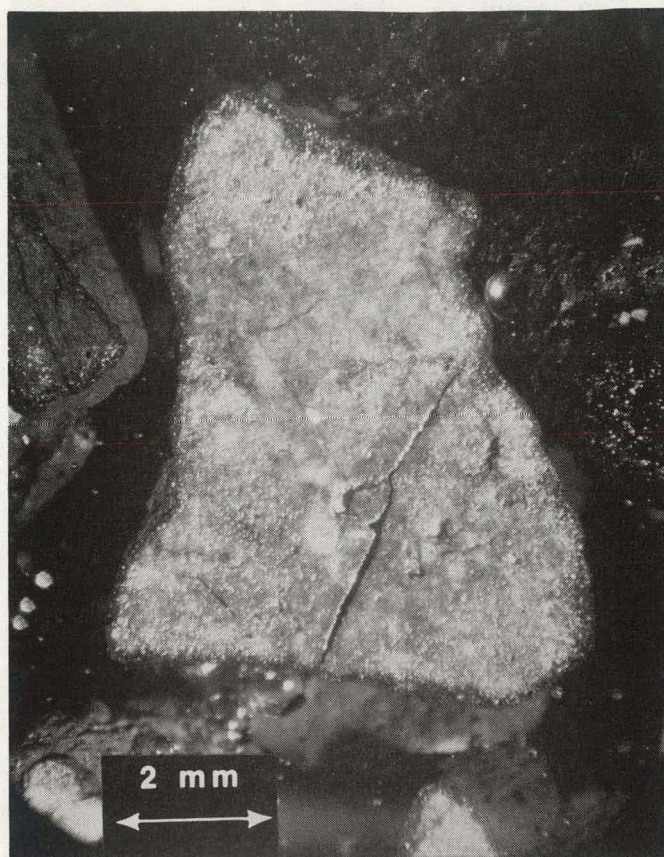
Figure 4. PHOTOMICROGRAPH OF CROSS-SECTION OF A SHALE PARTICLE WITH AN IRON-RICH COATING IN THE VENTURI DISCHARGE FROM RUN 122
