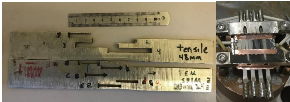
Figure 8. (a) Location of tensile bars and TEM specimens from a slice of the SAS508-304L weldment and (b) tensile bars and TEM specimens mounted onto the ion accelerator sample stage.
