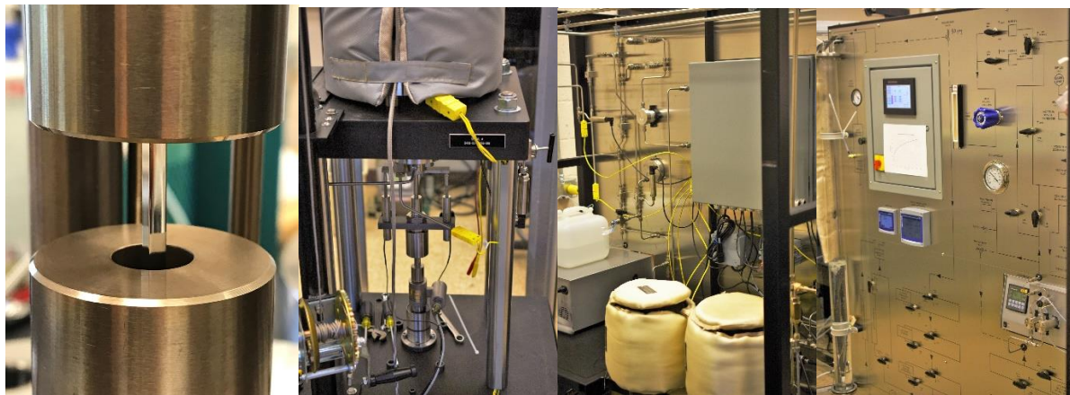
Figure 13. Left to Right: Tensile specimen (not a SCC tensile bar) mounted on the autoclave load frame grips; load frame strain gauges and load cell below the autoclave pressure vessel; autoclave loop hardware and preheaters (foreground); front of the loop stand with the water column, showing water flow control valves, high pressure pump, high pressure control valve (blue), and water analytics.
