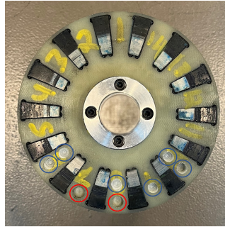
Fig. A11.4: Balancing holes drilled in the rotor housing. In addition to the original two static balance holes (red circle), four holes were added to achieve dynamic balance.
