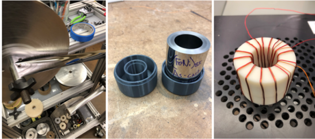
Fig. A5.6: Core winding and testing of 50 mm wide ribbon.
