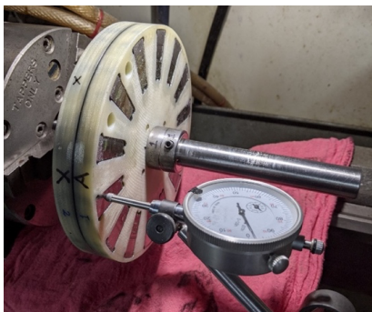
Fig. A11.2. Rotor face stiffness and runout measurements.
