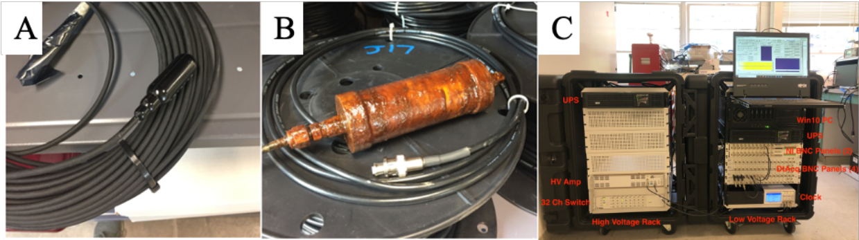
Figure 11. Pictures of a hydrophone (A), Piezoelectric Source (B), and the CASSM control system.
