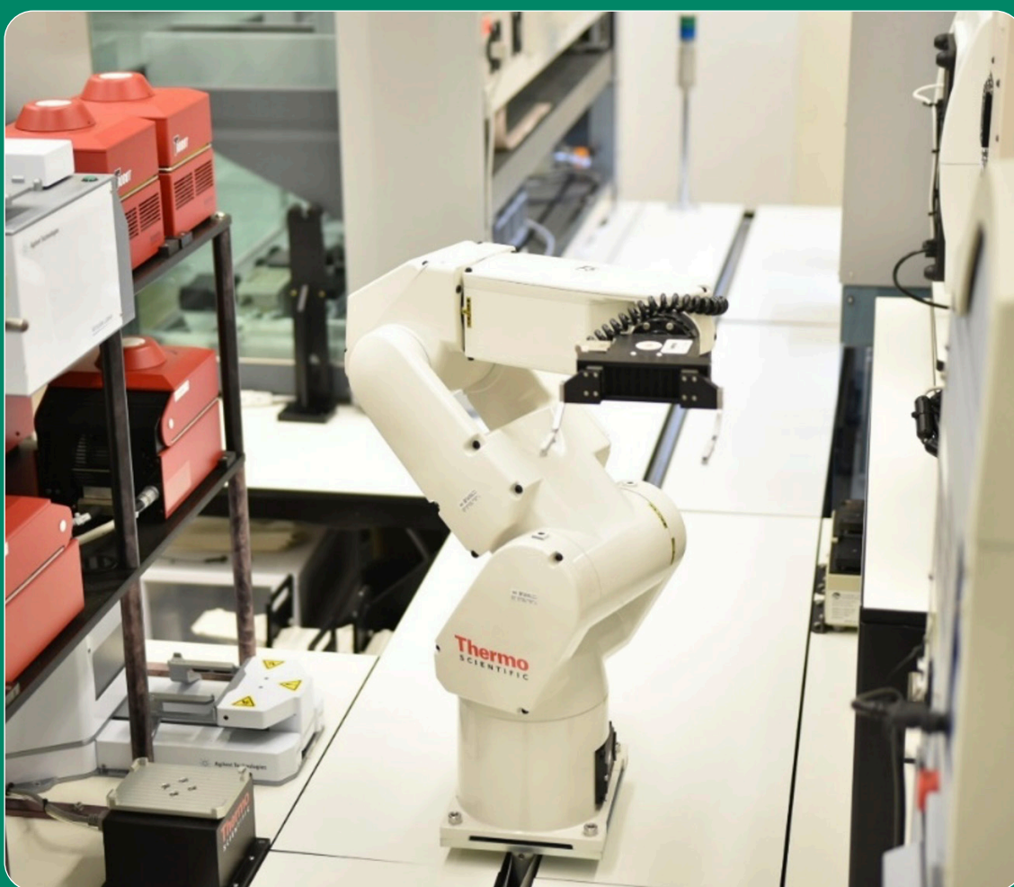
BioAutomata: An Integrated Robotic System for Autonomous Experimentation Driven by Artificial Intelligence and Machine Learning (AI/ML). The platform was developed by researchers from DOE's Center for Advanced Bioenergy and Bioproducts Innovation (CABBI). [Courtesy CABBI]
