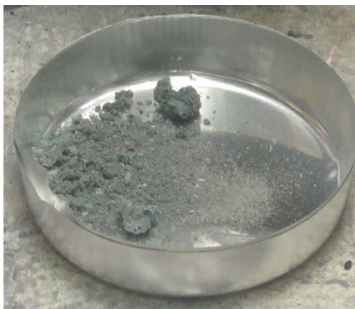
Figure 3. Photograph of the chlorinated plutonium product.
