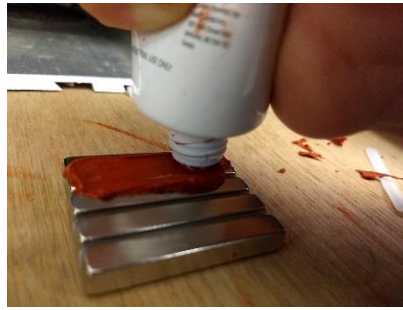
Adhesive applied in rows to completely fill gaps
