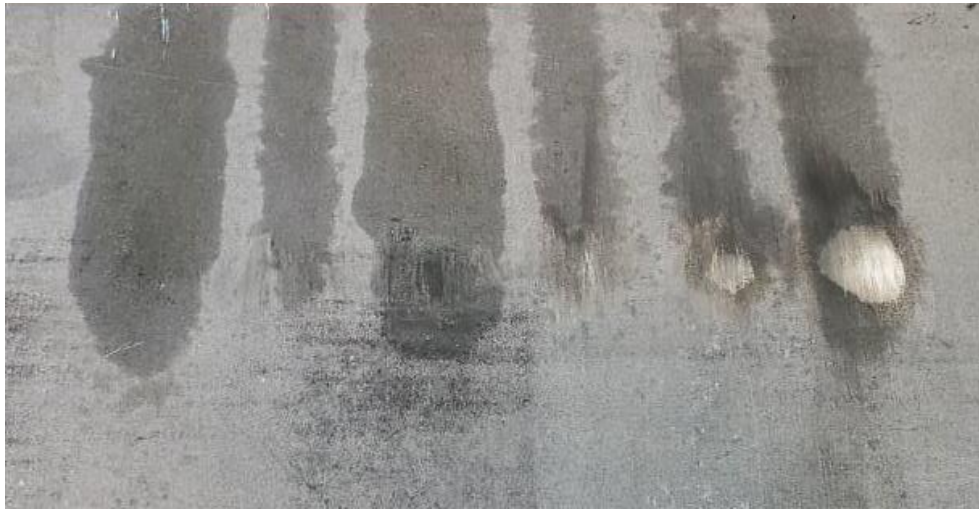
Figure 103: Brush system removing mill scale from an A36 steel plate.
