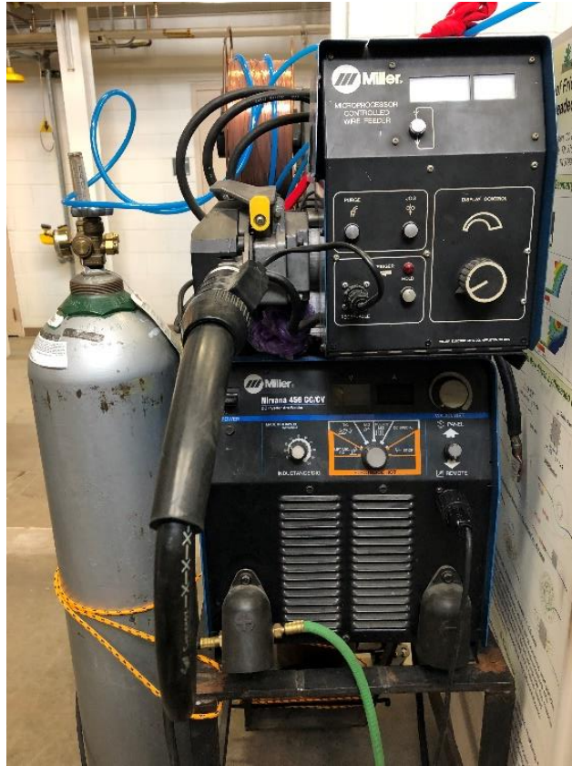
Figure 65: The TIG preheating setup.
