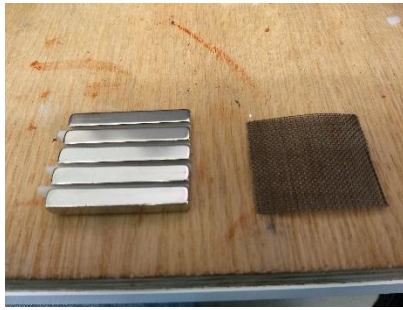
Magnets arranged, cloth cut & surfaces cleaned with xylene
