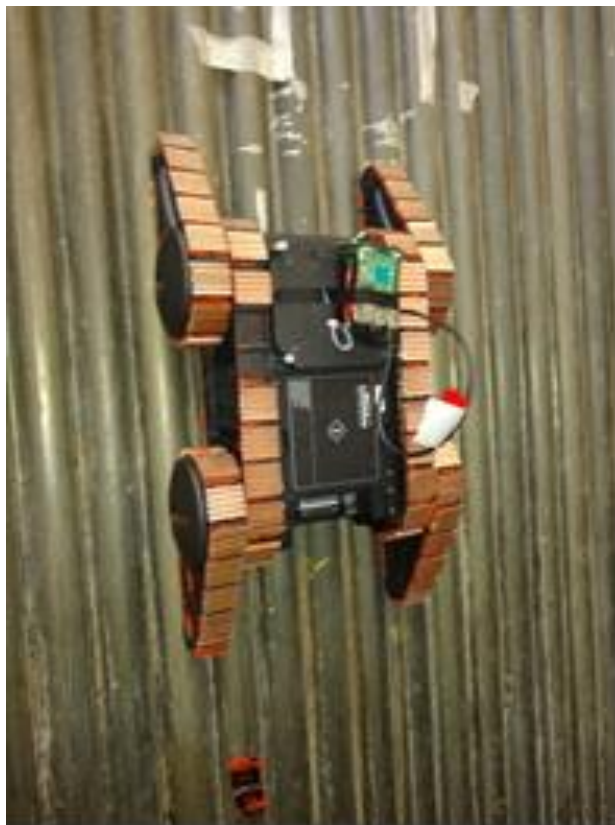
Figure 95: The robotic platform has been demonstrated traversing a vertical waterwall using magnets for attachment.
