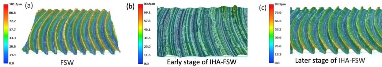
Figure 80: Surface morphology of (a) FSW and IHA-FSW trial 1 (b) early stage and (c) later stage.
