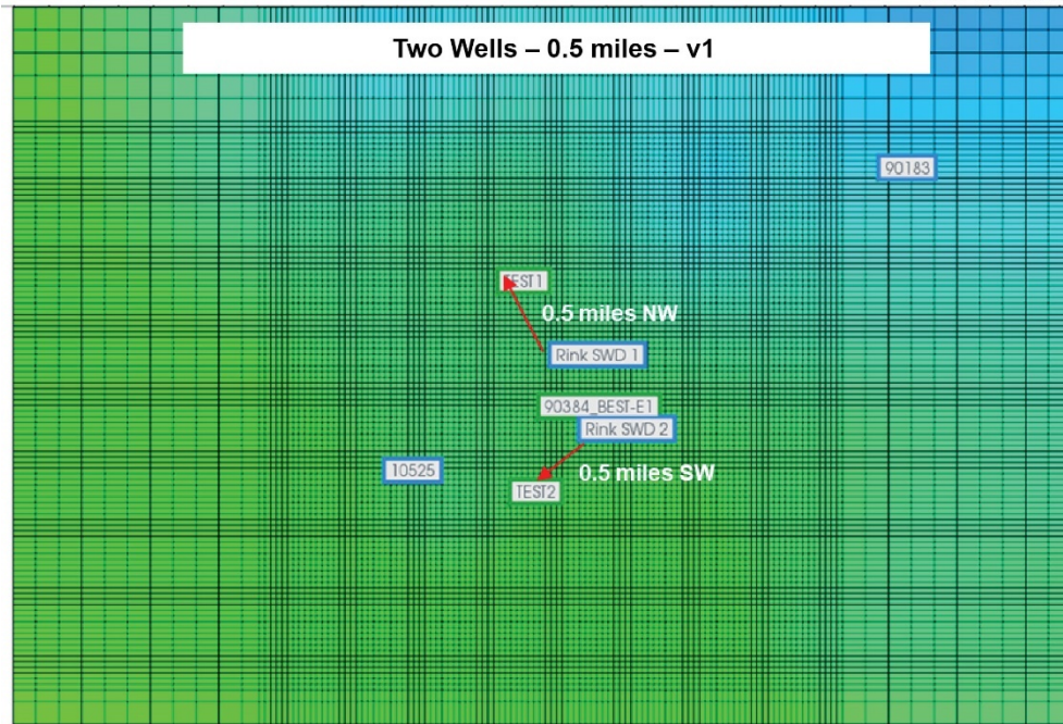
Figure D-1. Field numerical model showing the location for two production wells and the distance from the wells to Rink 1 and 2 SWD wells – Scenario 2 (a and b).
