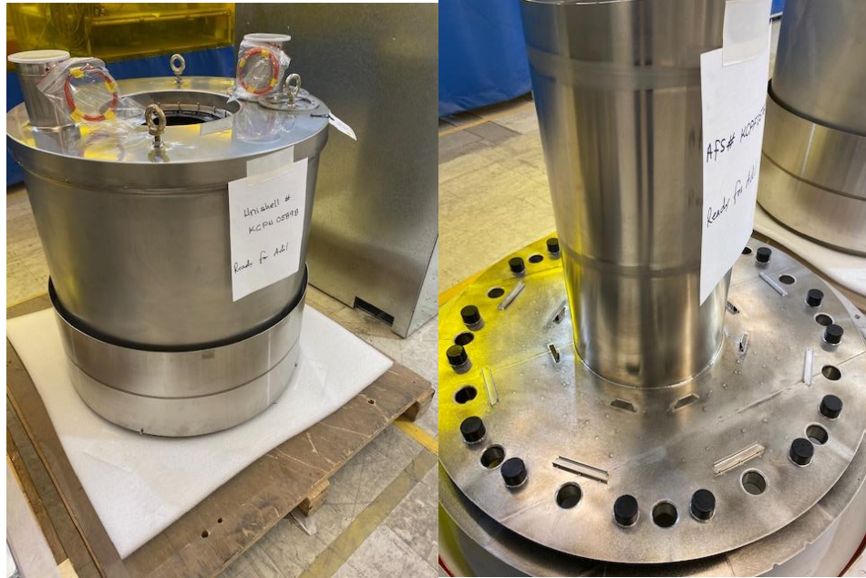
Figure 190 two major subassemblies for one of the hotbox
