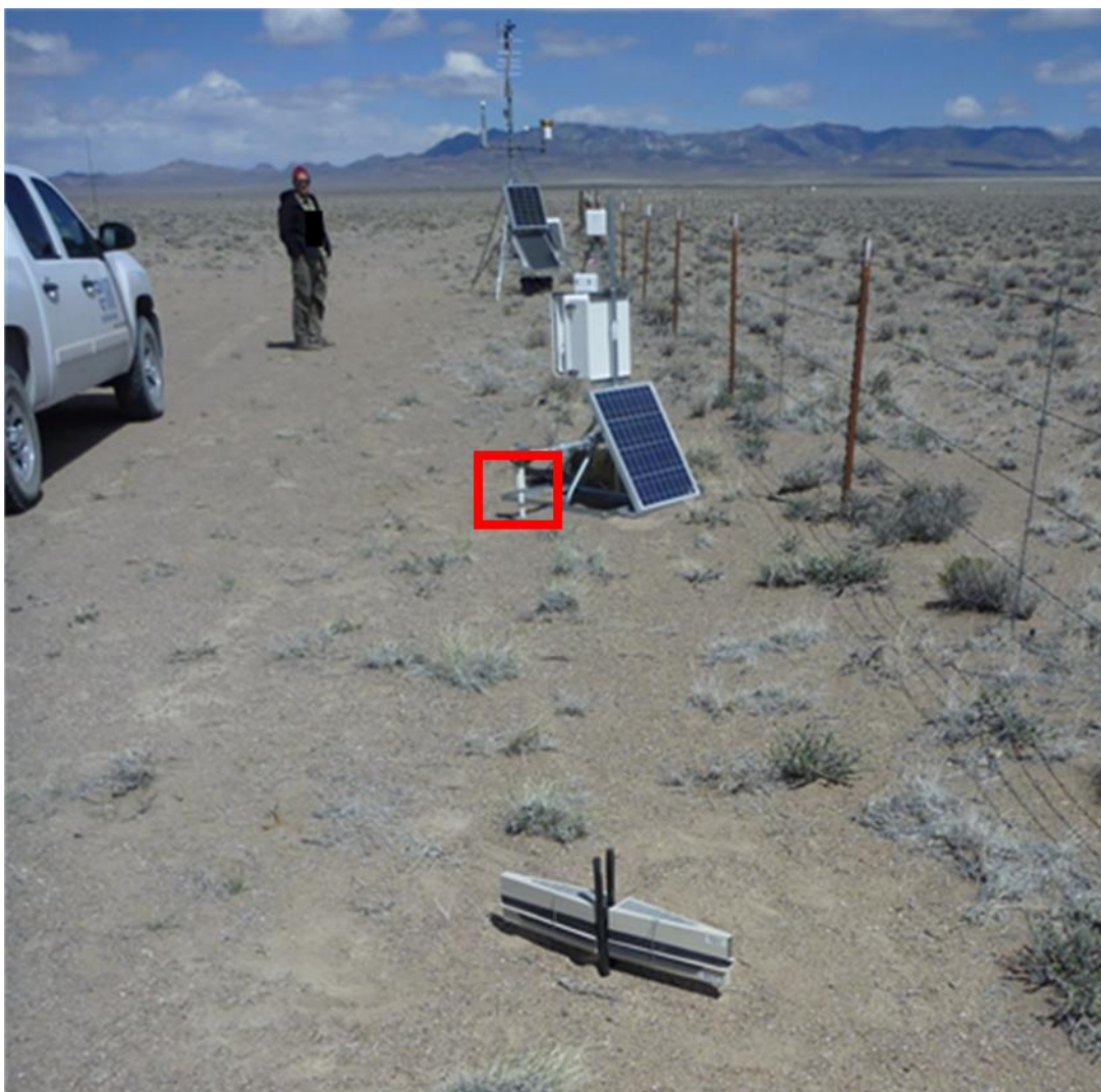
Figure 5. Northeast view at Station 401 prior to station relocation. In the foreground is one of three BSNE sand trap installations at this station. The Clean Slate III boundary fence is to the right. Behind the sand trap is the Sensit saltation sensor (highlighted by the red box) and a meteorological station with additional sand traps (not visible) is located along the fence line.
