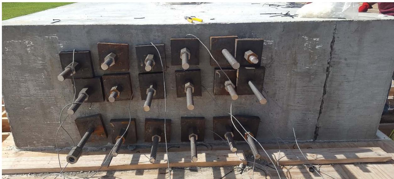
Figure 65 Specimen 2- Post-Tensioning Bars with Anchor Plates and Nuts, Side View
