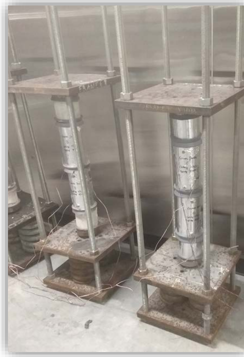
Figure 21. Uniaxial concrete creep test setup.
