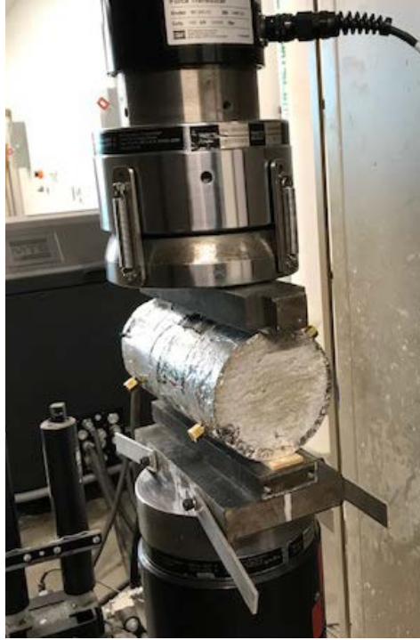
Figure 31. Experimental set up of splitting tensile test.
