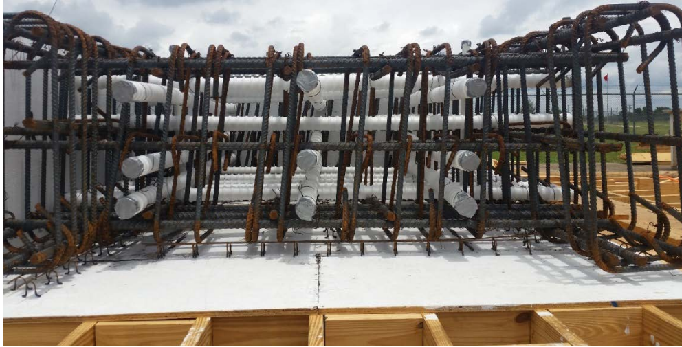
Figure 63 Specimen 2- Post-Tensioning Bar Ducts, Reinforcing Steel Cage, and Formwork View from Between Specimen 2 Feet
