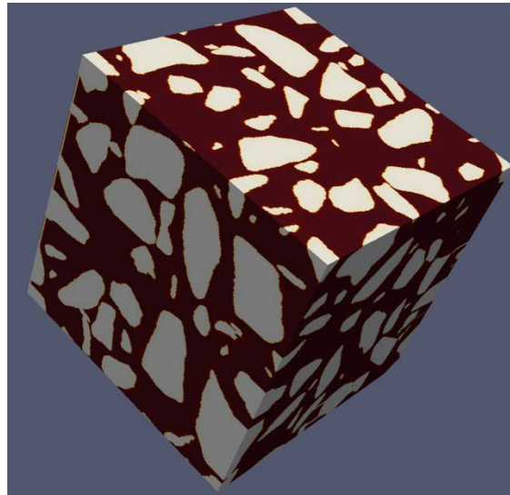
Figure 36. Completed three-dimensional microstructure containing 38% volume coarse aggregate, generated with periodic boundary conditions
