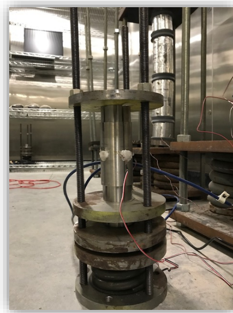
Figure 14. Confined creep test setup using the miniaturized creep frame placed inside an environmental chamber maintaining constant temperature and humidity.
