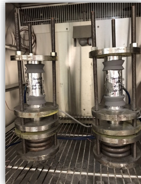
Figure 7. Uniaxial creep test setup using the miniaturized creep frame inside an environmental chamber maintaining constant temperature and humidity.
