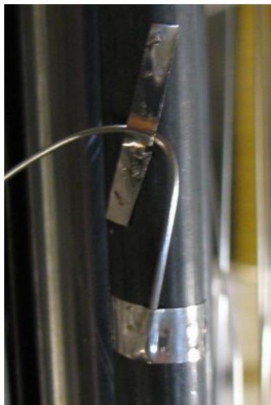
Figure 2.4 Typical TC attachment to heater rod.
