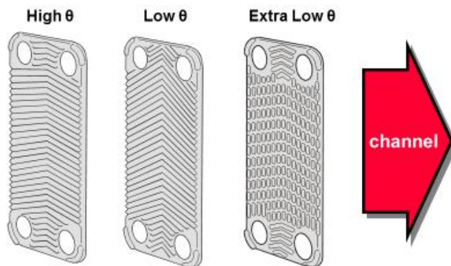
Figure 14. Differing plate geometries. High \Theta represents better heat transfer per unit of surface area, but has a greater fouling tendency. Extra low \Theta has lower heat transfer per unit of surface area, but has a lesser tendency to foul [7].
