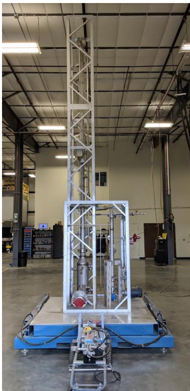
Figure 70. Fully assembled distillation column before adding side panels and loose perlite insulation.
