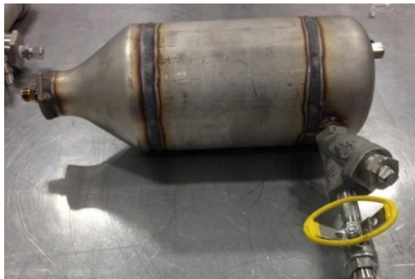
Figure 73. One of the pollutant settling tanks with a vapor–liquid separation drain and filter on the bottom.
