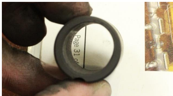
Figure 58. External gear pump bearing showing uneven wear, as evidenced by the thinner wall towards the upper right.
