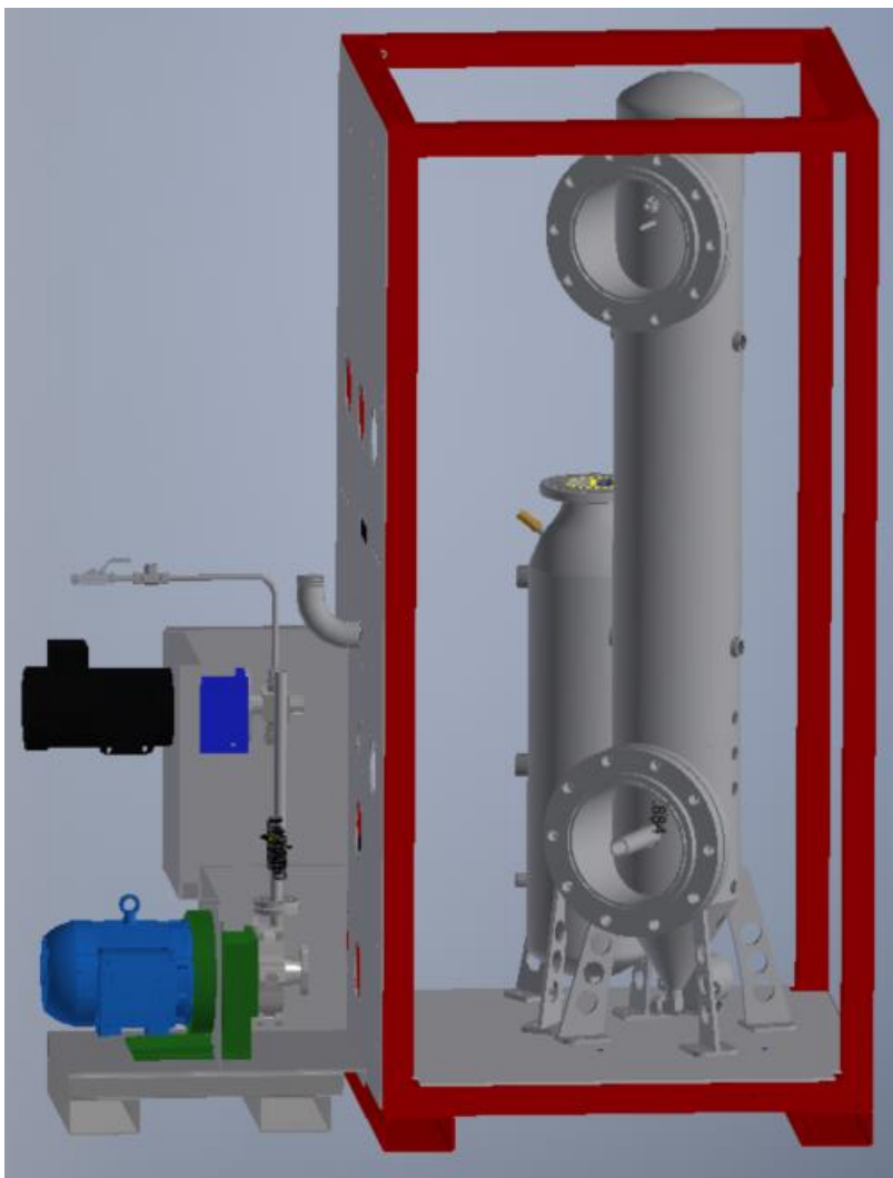
Figure 51. Drawing of the spray tower coldbox. The vessel in the front on the right is the spray tower. The vessel partially obscured behind and to the left is the vapor–liquid separator.
