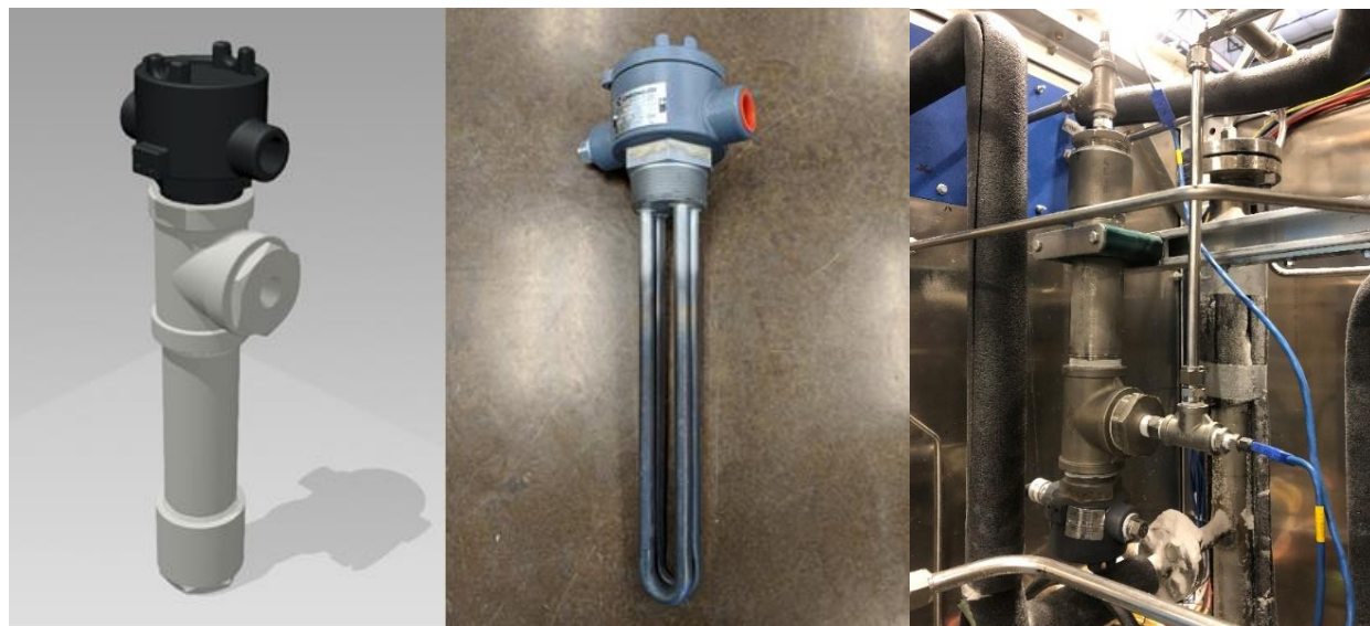
Figure 47. (left) Recuperator heater casing design, (middle) actual heater, and (right) installed.
