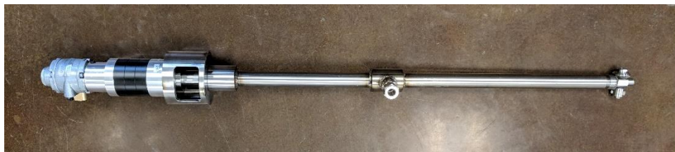
Figure 54. Spray nozzle assembly prior to mounting in the spray tower. The liquid to be sprayed enters at the compression fitting in the center of the image. The air motor that turns the drive shaft is on the left and the spray head and drive gear is located on the right.
