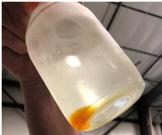
Figure 84. Sample of contact liquid chilled in a freezer to -40\text{ }^{\circ}\text{C} . The amber liquid is a separate liquid phase; its composition will be determined by future analytical tests.
