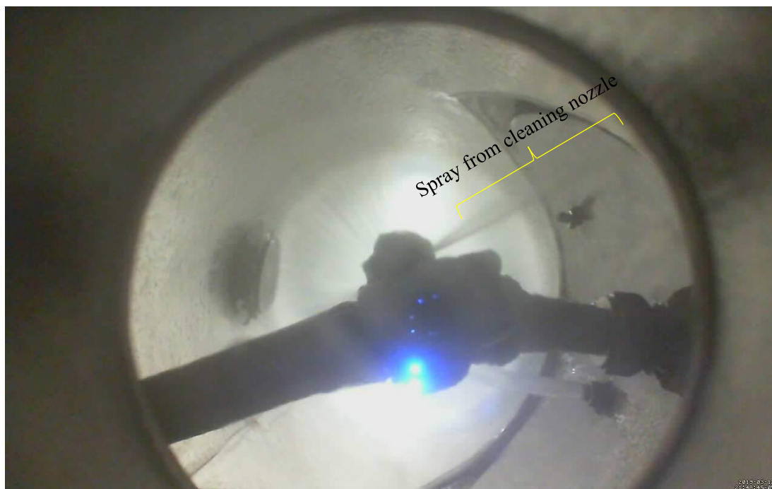
Figure 55. Interior of the spray tower showing the cleaning spray.
