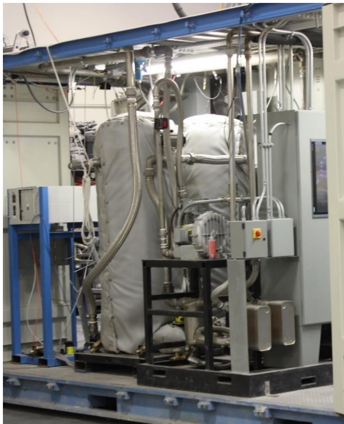
Figure 44. Mol sieve dryer integrated with the CCC ECL™ Skid. Both beds are covered with blankets of gray fiberglass insulation.
