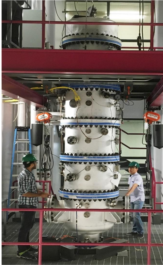
Figure 4-2 Photo of 100 kWth Pressurized Combustor of the SPOC Pilot Testing Facility
