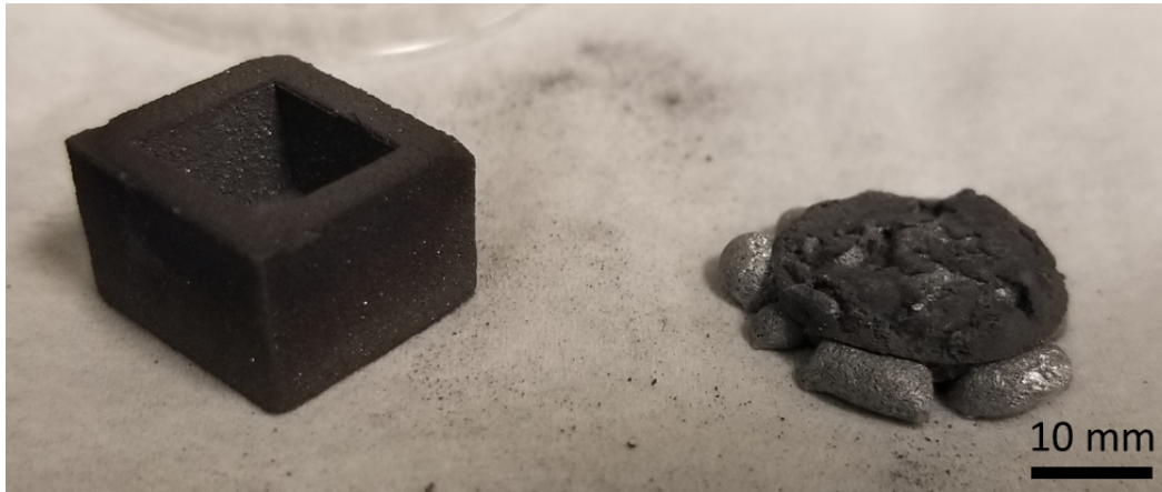
Figure 13. TiC preform infiltrated by NiAl 3 at 1000°C for 30 min. Material remnant (right) shows clear melting behavior and segregation of Al-rich phase.
