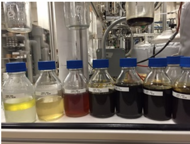
Figure 58: Photograph of the first batch of hydrotreated product collected in the first 30 hour run of experiment 1.
