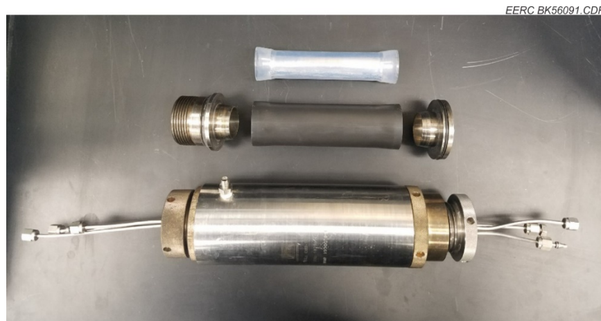
Figure 6. Inner gasket assembly and Hassler-style core holder.
