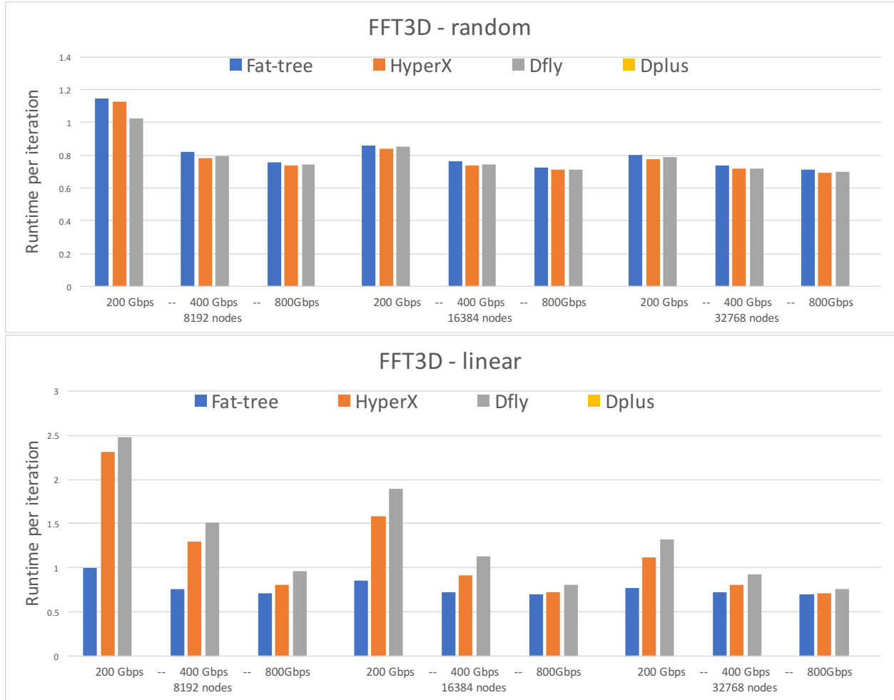
Figure 19: SST/merlin results for the FFT3D motif using both linear and random placement of ranks. Results are normalized to the 8192 node fat-tree with 200Gbps injection bandwidth results.
