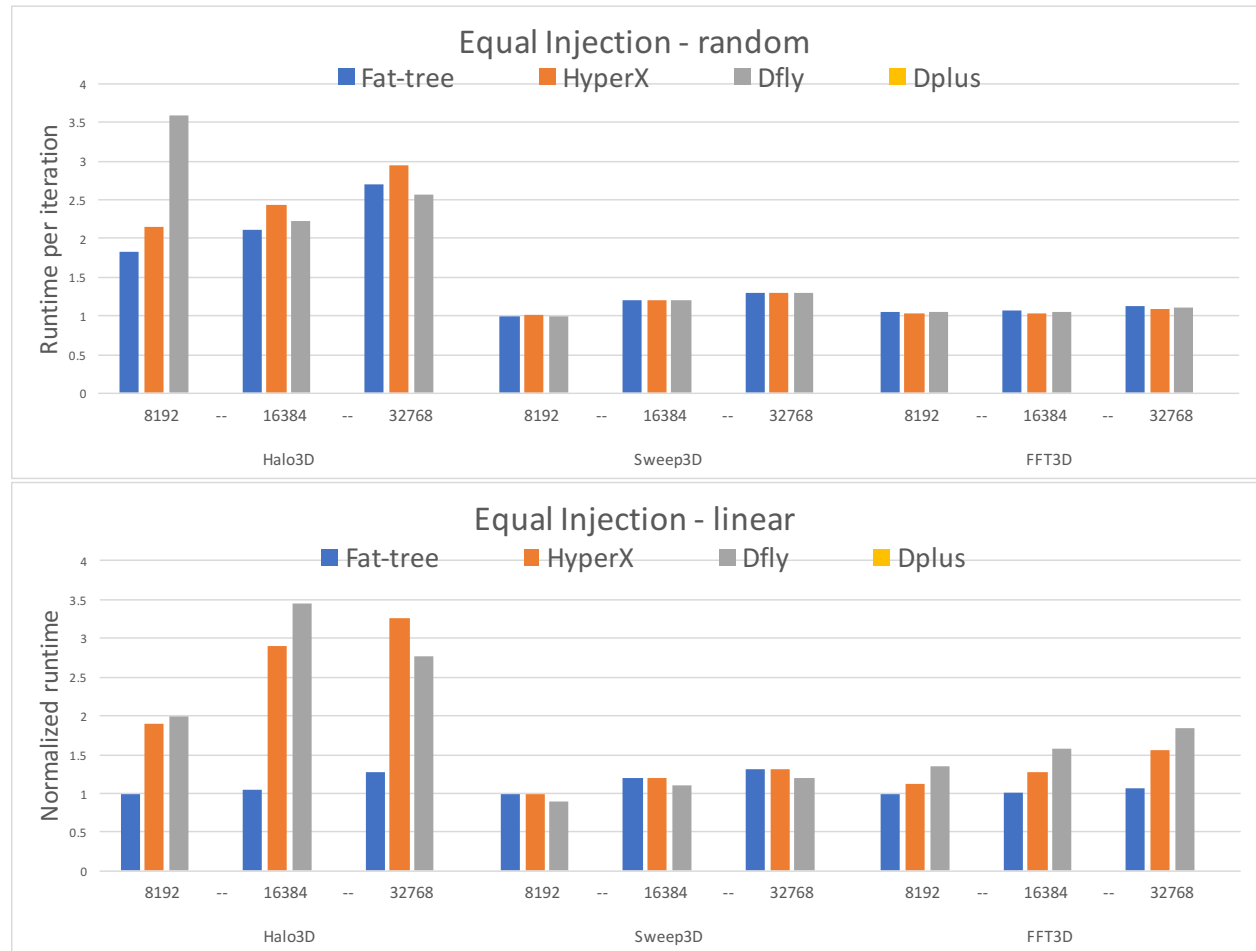
Figure 20: SST/merlin results comparing configurations with equal injection bandwidth per rank (8k/800 Gbps, 16k/400 Gbps and 32k/200 Gbps) for each of the benchmarks.
