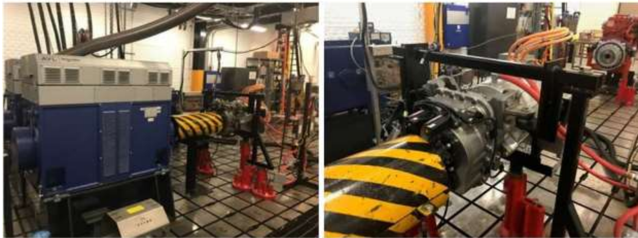
Figure 4. Eaton four-speed EV AMT and UQM Electric Motor on the HIL test setup at ORNL
