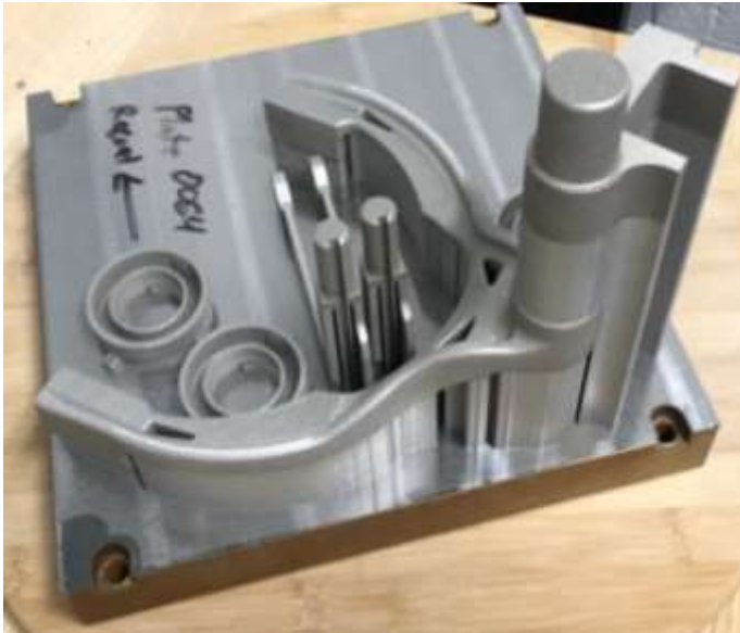
Figure 101. 3D-printed shiftbar assembly on the base plate and the support structure.
