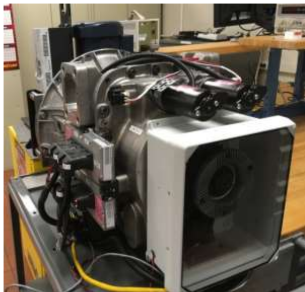
Figure 103. Transmission calibration and controls bench test setup
