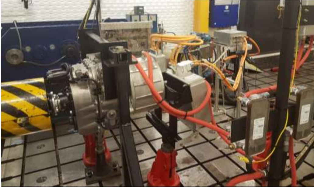
Figure 113. Electric powertrain system fully installed at ORNL's VSI Powertrain Test Facility
