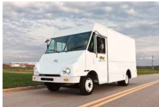
Figure 9. Newton Step Van, 16,500 lb GVW (7.5 t), Class-4.
