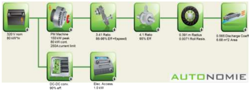
Figure 32. Autonomie representation of battery electric medium-duty truck architecture
