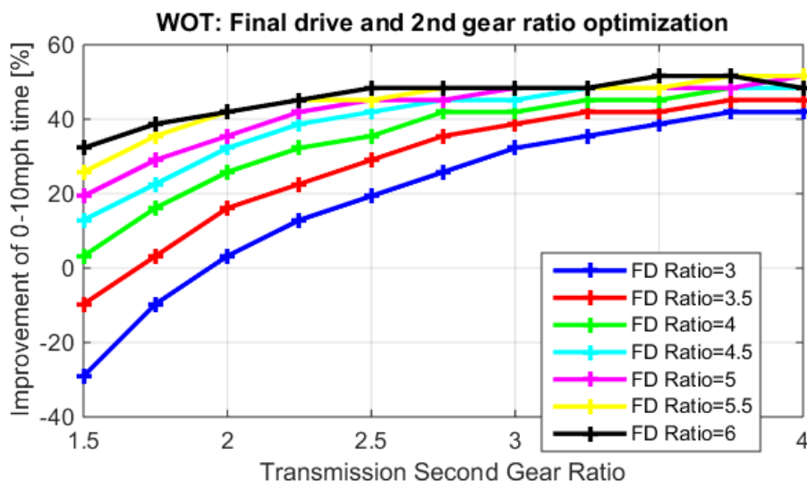
Figure 62. Final drive ratio and the second gear ratio effect on 0-10mph acceleration
