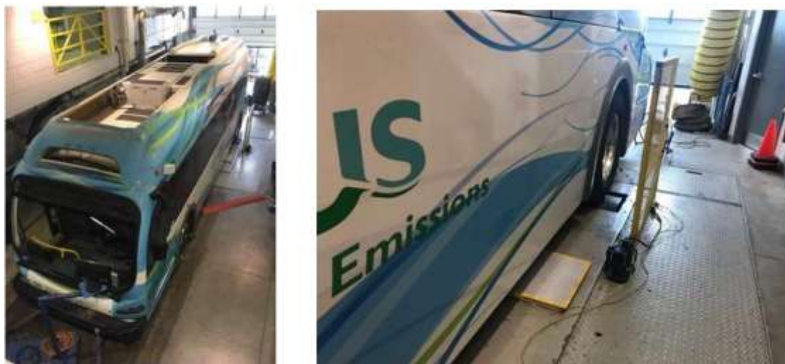
Figure 6. Vehicle mounted on NREL's heavy-duty chassis dyno with all data acquisition implemented and ready for testing
