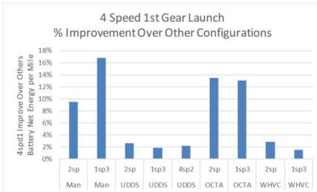
Figure 7. Efficiency improvement verification test results on NREL's HD chassis dyno. This chart does not include the efficiency gains due to the FDR change from 9.8 to 6.2.
