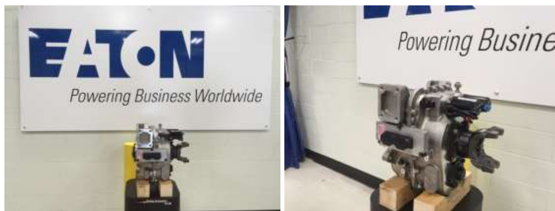
Figure 95. The display unit of the new four-speed EV Transmission.
