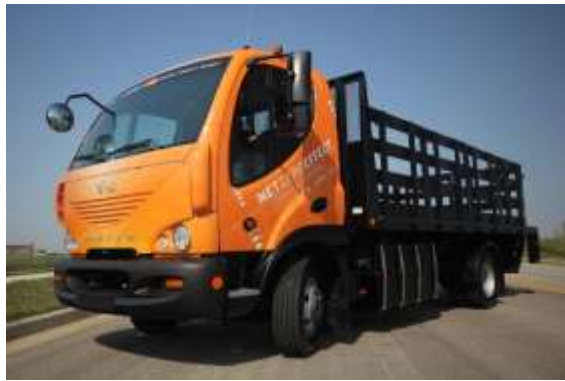
Figure 8. Newton Cab Chassis, 22,000 lb GVW (10 t), Class-6.
