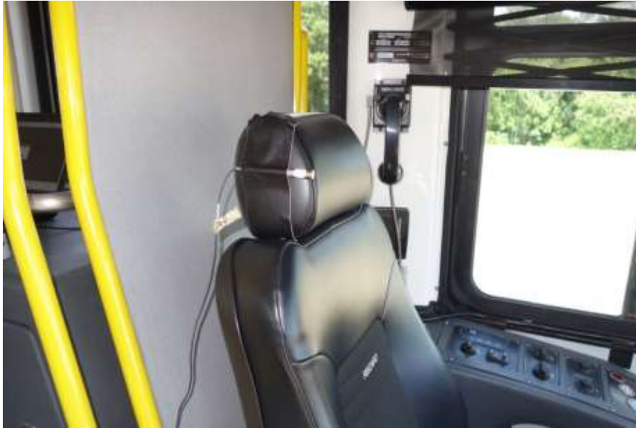
Figure 130. Vehicle noise measurement setup at driver seat
