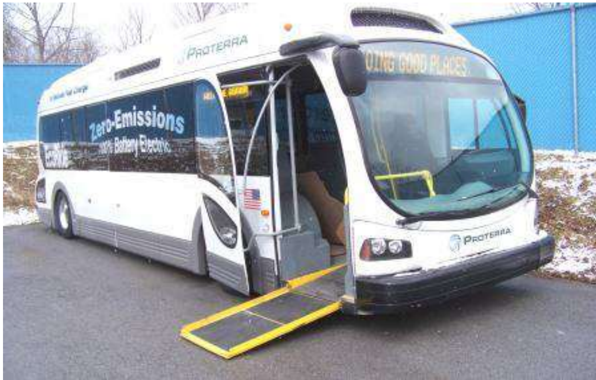
Figure 81. Proterra BE35 Electric Transit Bus equipped with two-speed Eaton transmission and a Lift-U-Model Lu-11-12-05 fold-out handicap ramp.
