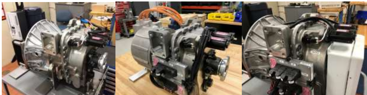
Figure 97. Three fully functional prototypes of the new four-speed EV transmission.
