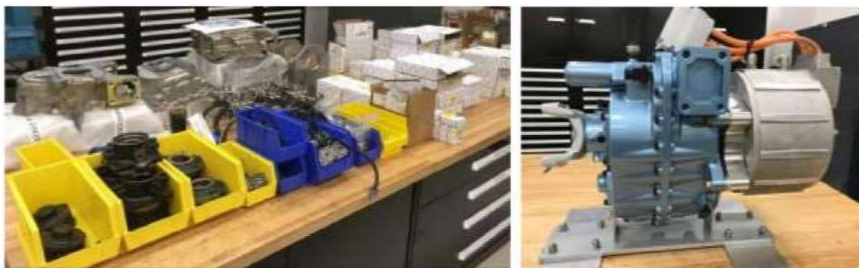
Figure 2. Left: Components of four-speed AMT are laid out before the assembly. Right: Eaton four-speed EV-AMT display unit integrated with a UQM Electric Motor.
