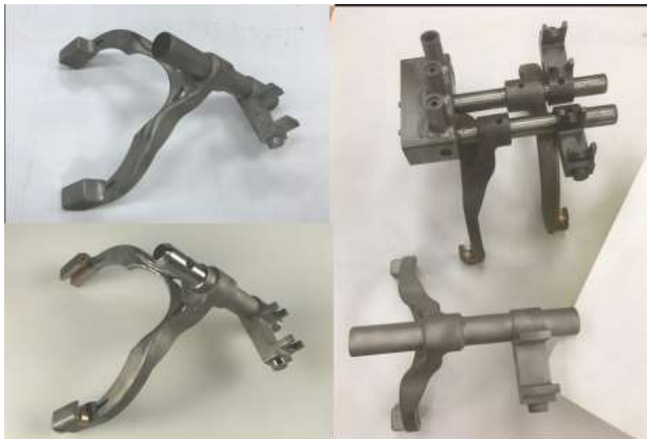
Figure 102. 3D-printed shiftbar assembly separated from the support structure.
