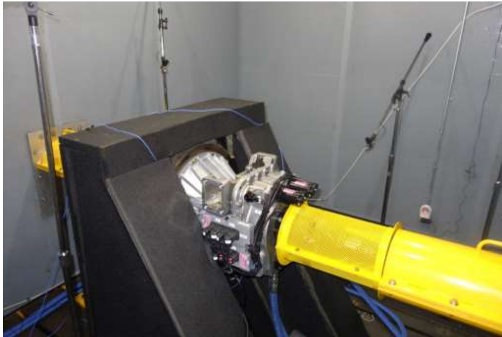
Figure 104. Transmission NVH setup
