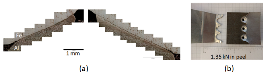
Figure 14. (a) Weld cross sections of spot weld with countersink target. (b) Top view of peeled sample with three weld spots.
