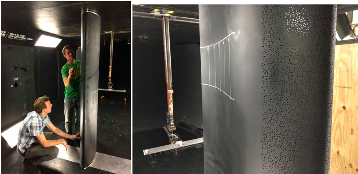
Figure 3.9. S814 airfoil model positioned in test section of tunnel and image of 15% distribution density roughness pattern applied to the leading edge, wake rake also visible in images.
