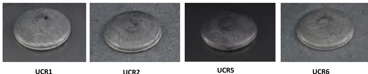
Figure 104: Round boss UCR formed heads for material/coating configurations UCR1, UCR2, UCR5, and UCR6
