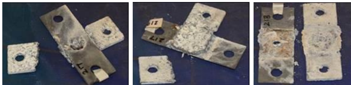
Figure 35: UPJ8-1 cross-tension test coupons separated after 8-wks of accelerated corrosion
