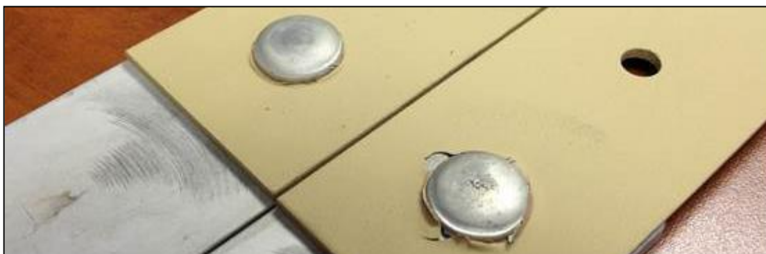
Figure 73: Photo of two joined lap-shear tension assemblies utilizing the CARC coating on the steel coupons
