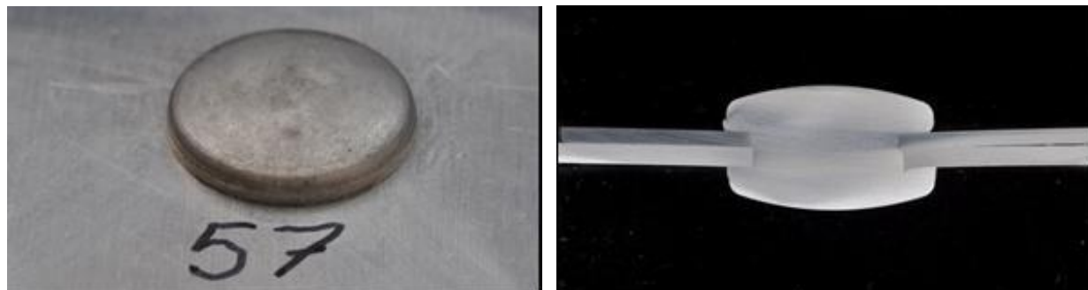
Figure 103: UCR head formation and metallographic cross section produced from optimized parameters
