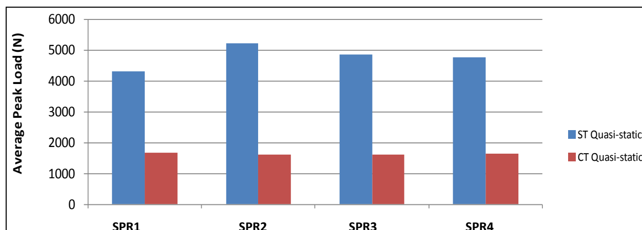
Figure 3: Quasi-static shear tension and cross tension test results for selected coating configurations of Mg AM60B to Al6013 SPR joints
