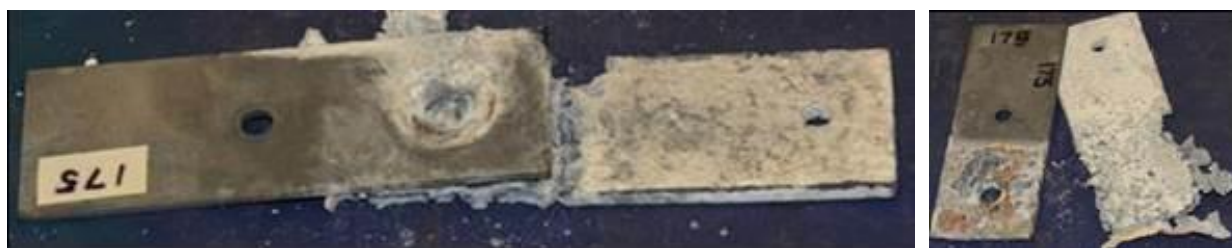
Figure 34: UPJ8-1 lap shear tension test coupons separated after 8-wks of accelerated corrosion
