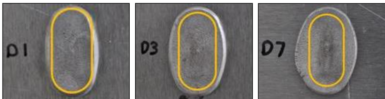
Figure 89: Effect of force and current on head shape and size
