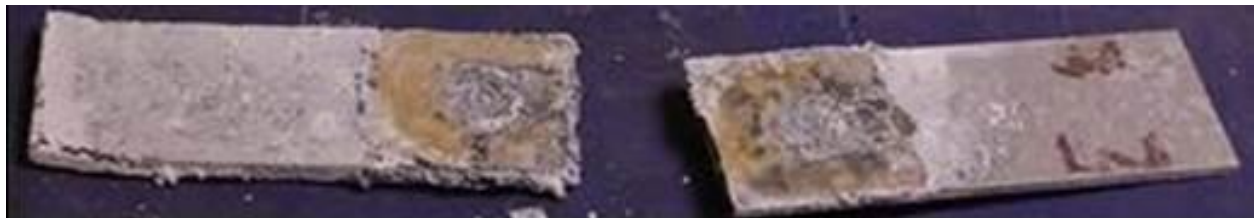
Figure 30: UPJ 8-2 Bare Mg to bare Al joint separation after 6 weeks
