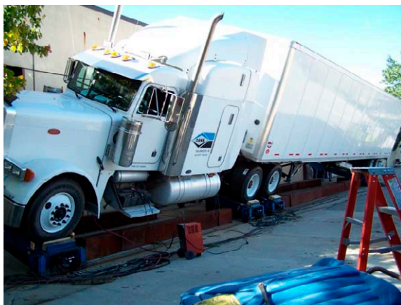
Figure 3.2.1 Test Vehicle on Tilt-Table.
