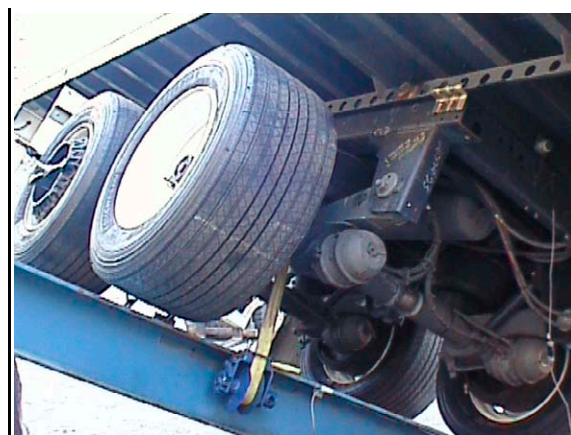
Figure 3.2.2 Trailer Axle 4 at Liftoff.
