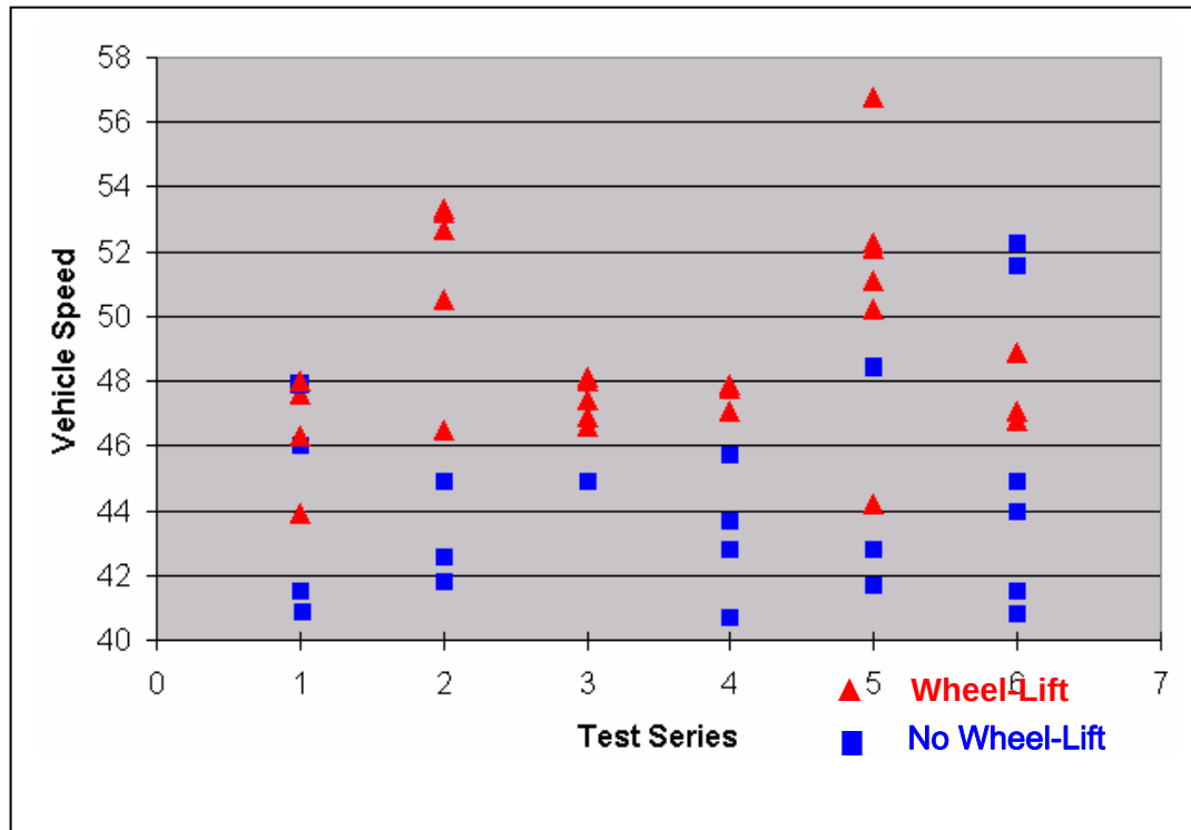
Figure 5.2.1 Vehicle Speed (mph) at Wheel Lift.
