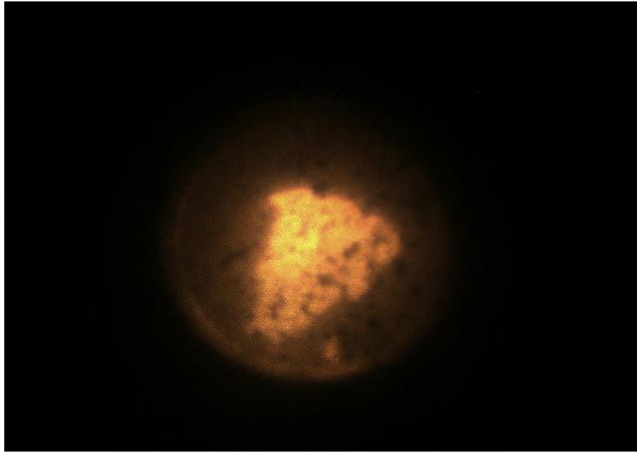
Figure 38. Sapphire window condition (Original design) after 5 weeks of testing under the previous project
