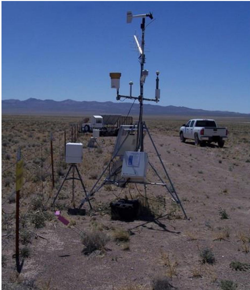
Figure 4. The solar powered air sampler, saltation sensor, and meteorological tower (background, center, and foreground, respectively) at Station 401 are located along the north fence that bounds the Clean Slate III contamination area.
