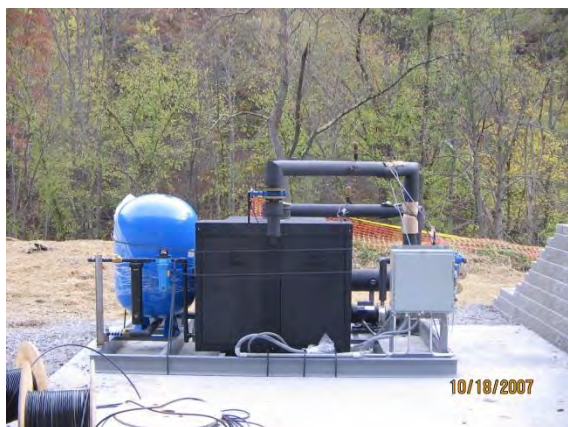
Figure 21. CO 2 vaporizer skid with the hot water boiler in the foreground.
