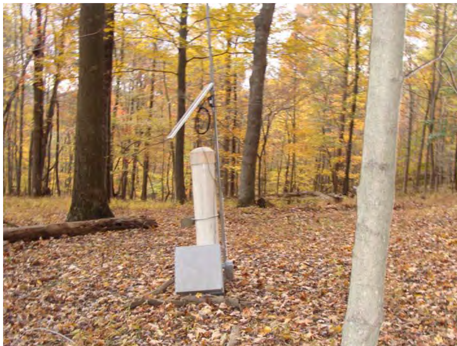
Figure 28. A tiltmeter monitoring location at the project site (photo courtesy of H. J. Siriwardane & R. K. Gondle, WVU).
