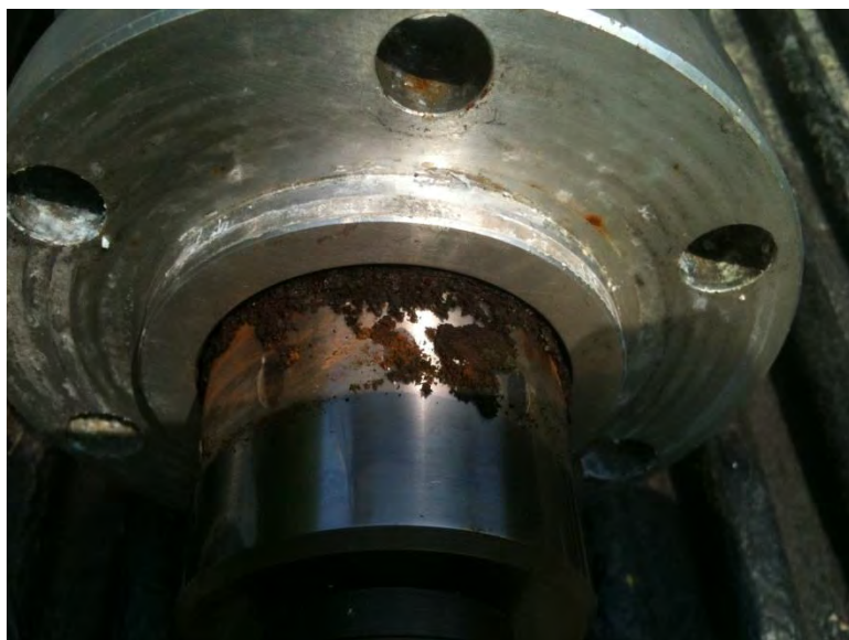
Figure 33. Accumulated debris with wear on an original pump cylinder and seal.
