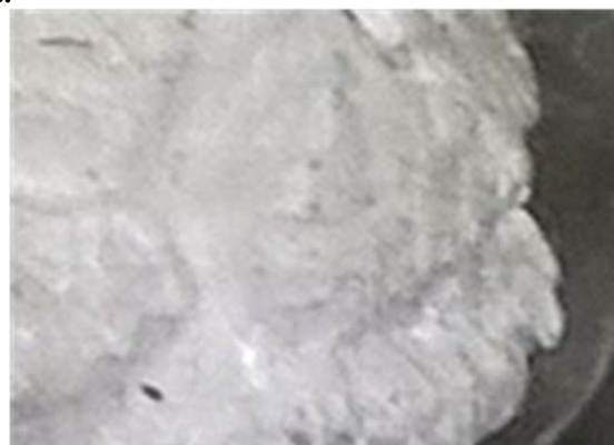
Figure 16. PS/POLYMER-BLEND-B/MMT-ABU foamed in pressure vessel. Foam density ~50kg/m 3 .
