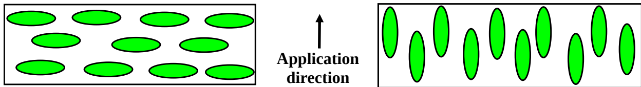
Figure 1. Spheroids aligned in-series (left), or in-parallel with the application direction (right). The left example (in-series) has a lower thermal conductivity (higher insulation value, or thermal resistance) than that of the right.
