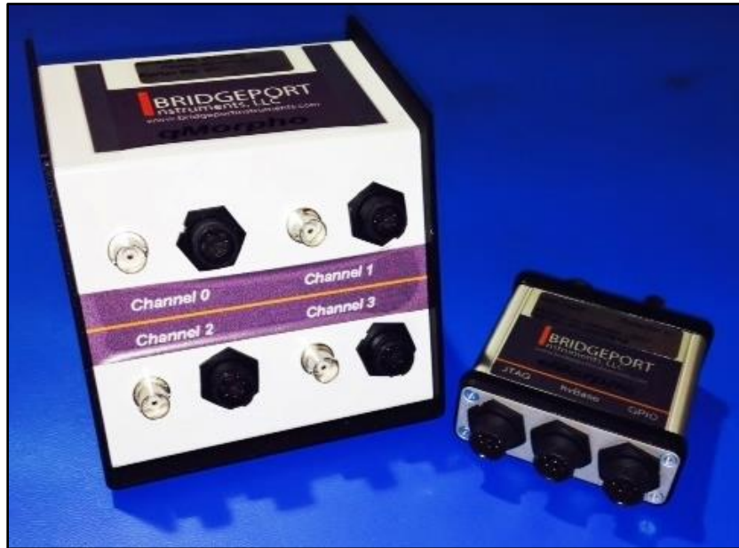
Figure 22 – qMorpho (left) and eMorpho (right) digitizers
