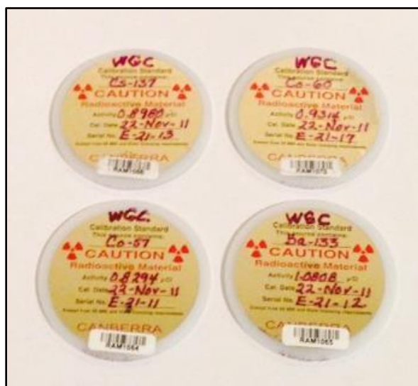
Figure 24 – Sealed gamma-ray check sources utilized in this study
