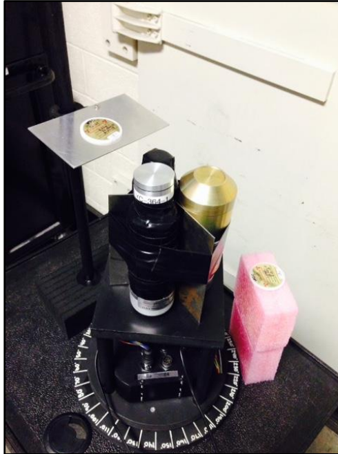
Figure 51 – Experimental setup for two source directional measurements
