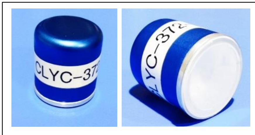
Figure 16 – Encapsulated 1-inch CLYC crystal used in experiments
