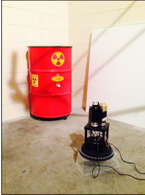
Figure 57 – Experimental setup for thermal neutron source directional measurements, R=1 m
