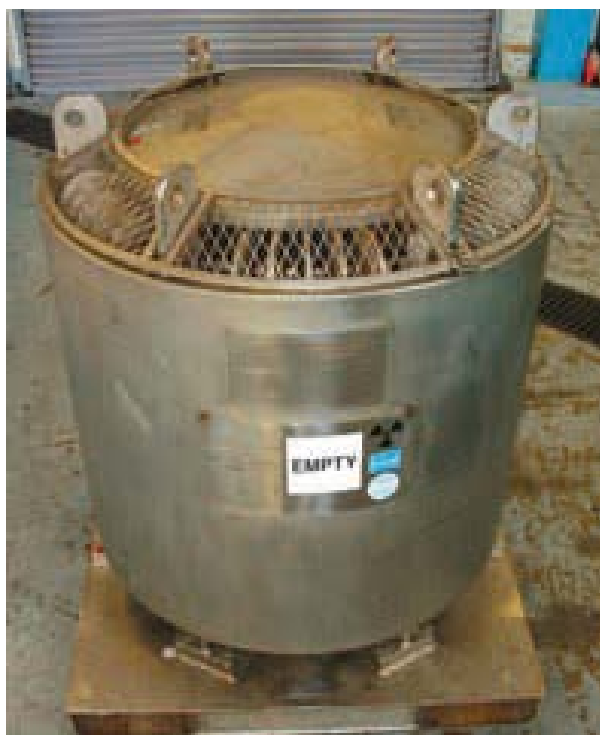
Figure 4: A high activity gamma ray source container in a shielded transport configuration 5 .
