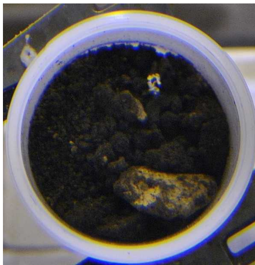
Figure 2. Photo of 105C-15-3, Through the Hot Cell Window, Showing Large Tan Aggregate Subsampled for Analysis.
