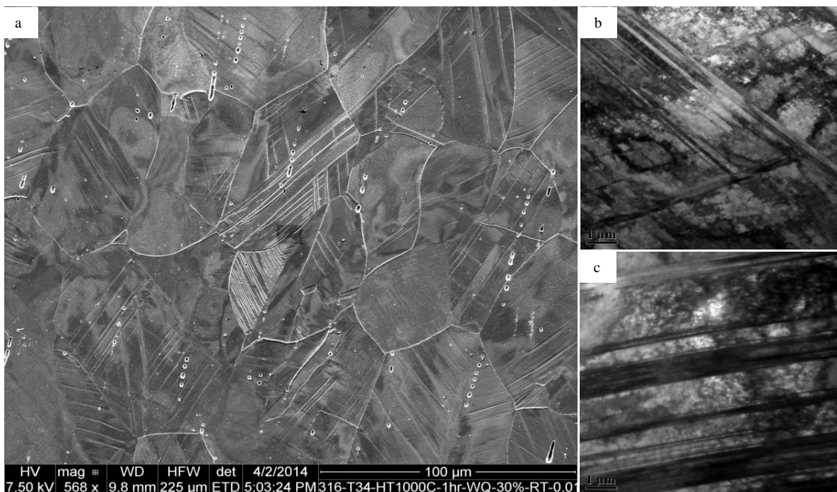
Figure 72 -316 Stainless steel annealed at 1000°C for 1 hour, uniaxial tension to 30% elongation, a) SEM image after etching, b and c) BF TEM images.
