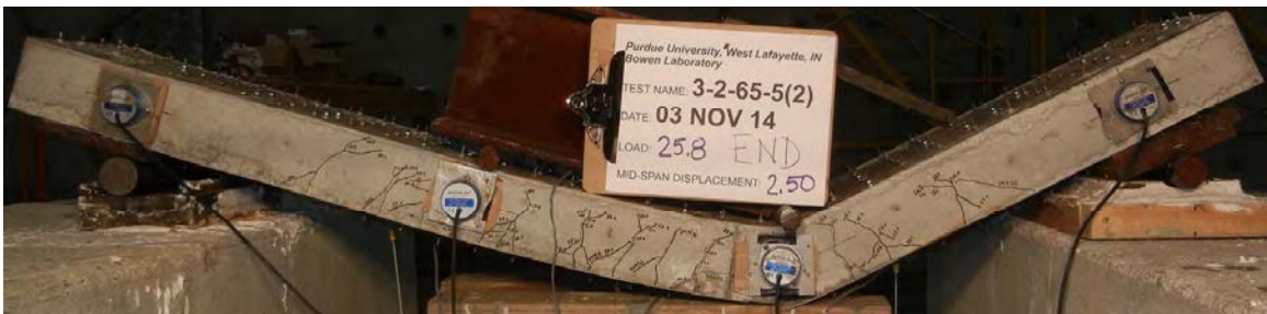
(b) Shear Cracks at Total Load of 20-kips
