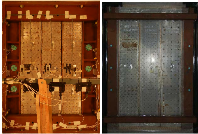
(a) View from Inside Target Vessel (b) View from Outside Target Vessel (Blast Face)
