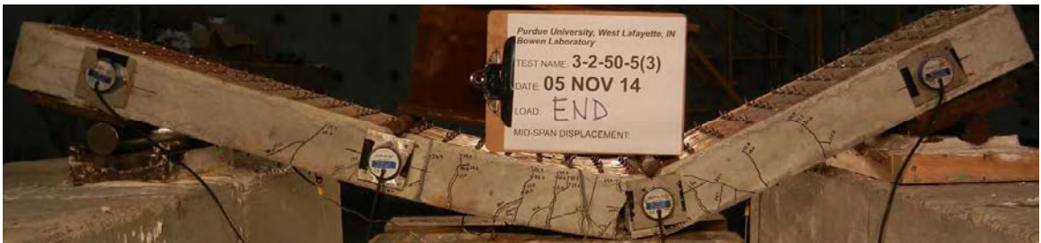
(b) Shear Cracks at Total Load of 20-kips
