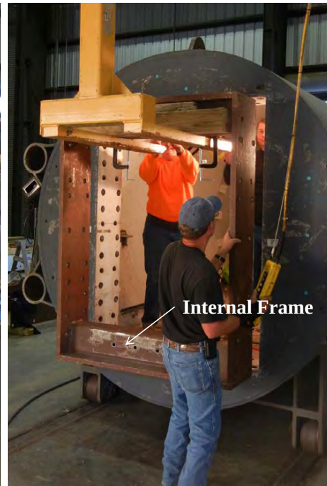
(b) Positioning Internal Frame
