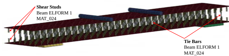
(b) Model With Concrete Removed
