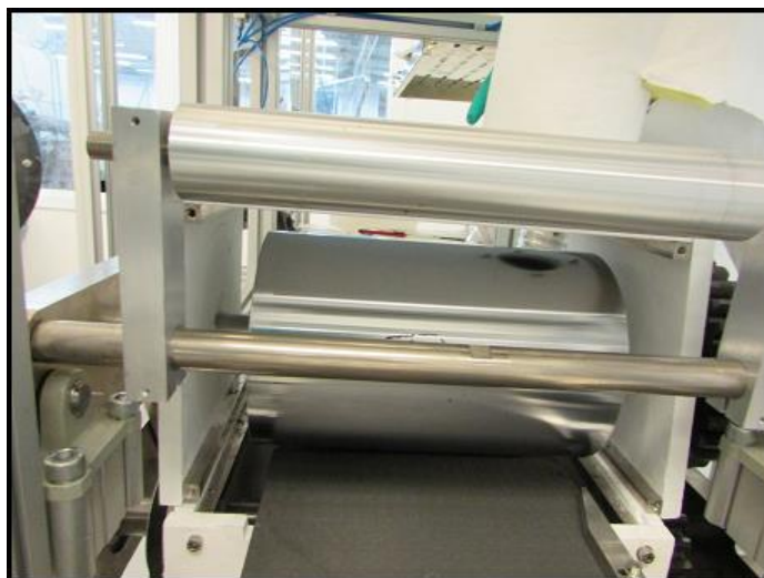
Figure 17: Pressing roller within the roll-to-roll machine
