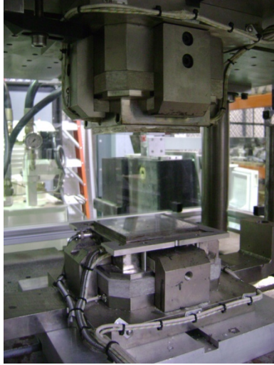
Figure 12: PMD precision thermal press modified for APC.
