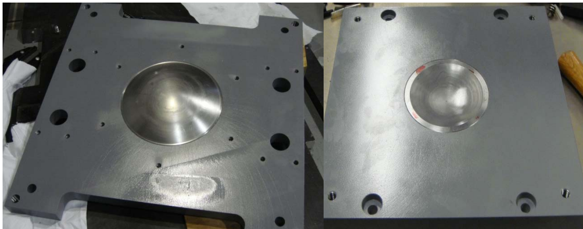
Figure 28: Matching spherical dome and seat are used to support the lower tooling. The geometry allows for a gimbal style alignment adjustment, but also supports high loads required during lamination.
