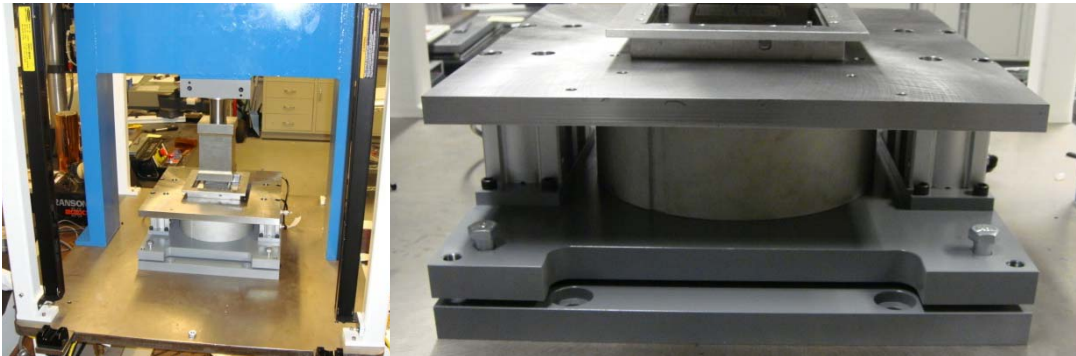
Figure 27: 15kHz ultrasonic lamination press. Bottom tooling is adjustable to obtain precision alignment after tooling assembly. H-Frame layout maintains tooling alignment.
