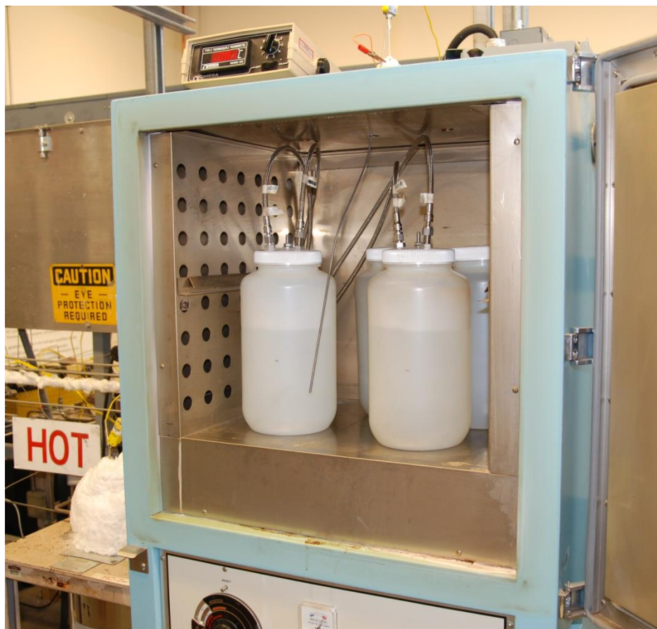
Figure 22 Humidification system for autoclave corrosion
