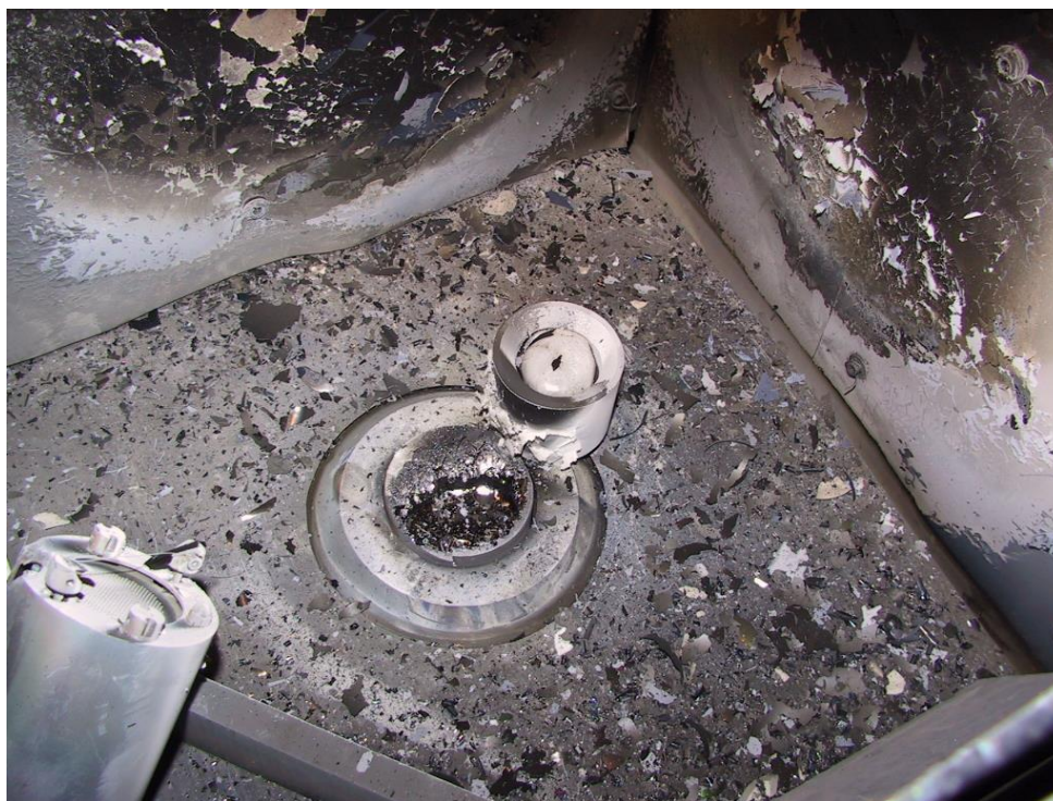
Figure 38. Evaporant sources after a mixed layer deposition.
